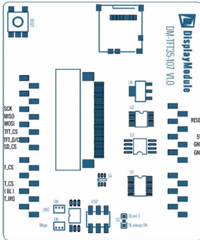
2.Pin function : This TFT panel connects directly on top of an Arduino pin compatible device.
