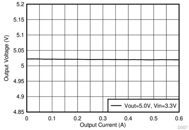
**Figure 9-22. Boost Output Voltage vs Load Current**
