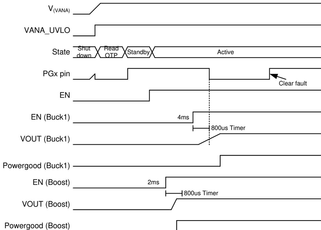
**Figure 8-10. PGx Pin Operation in Gated Mode.**
