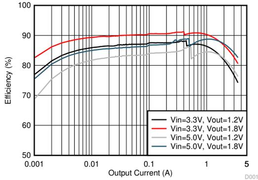
**Figure 9-3. Buck Efficiency in AUTO (PFM/PWM) Mode**
