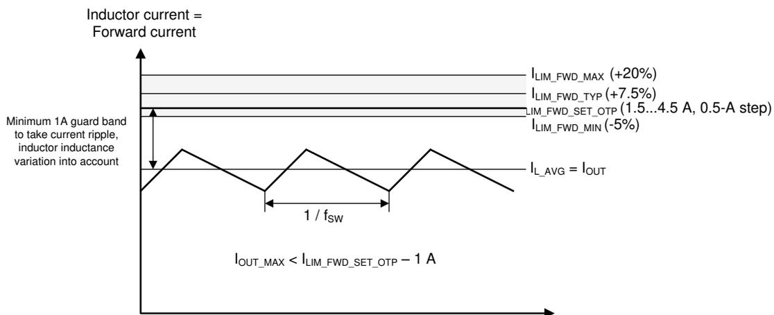
**Figure 9-2. Current Limit vs Maximum Output Current**
