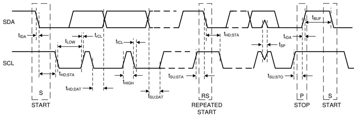
Figure 7-1. I<sup>2</sup>C Timing
