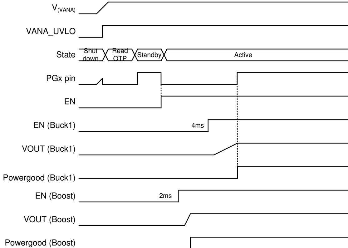
**Figure 8-11. PGx Pin Operation in Continuous Mode**
