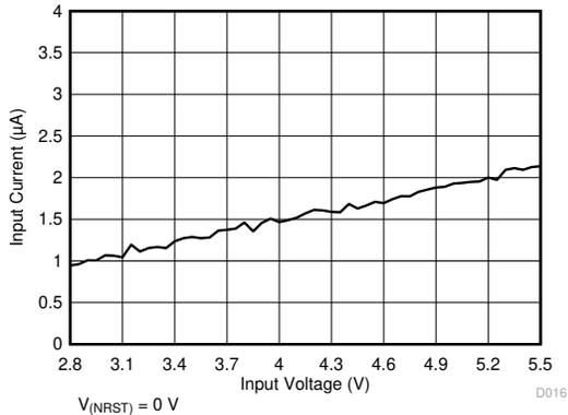
**Figure 7-2. Shutdown Current Consumption vs Input Voltage**
