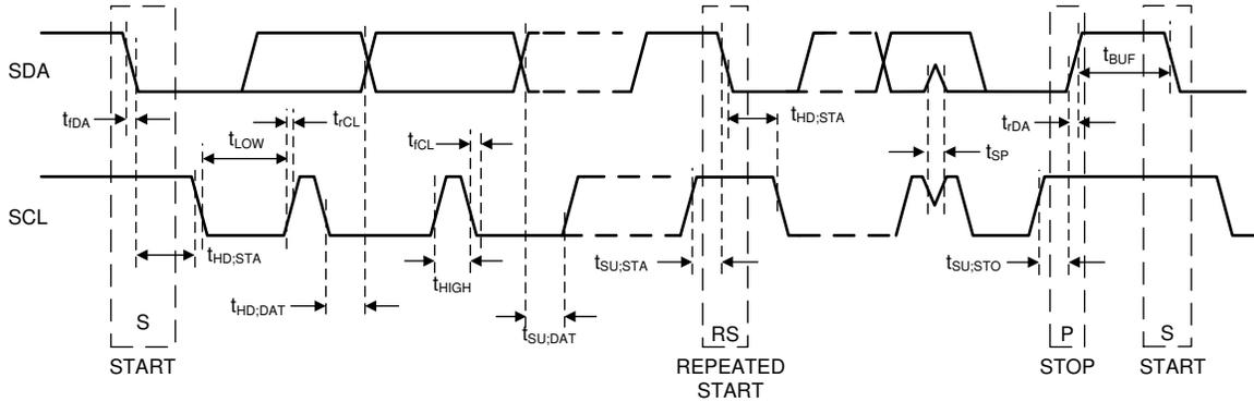
Figure 8-17. I<sup>2</sup>C-Compatible Timing
