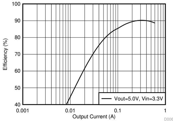
**Figure 9-21. Boost Efficiency**
