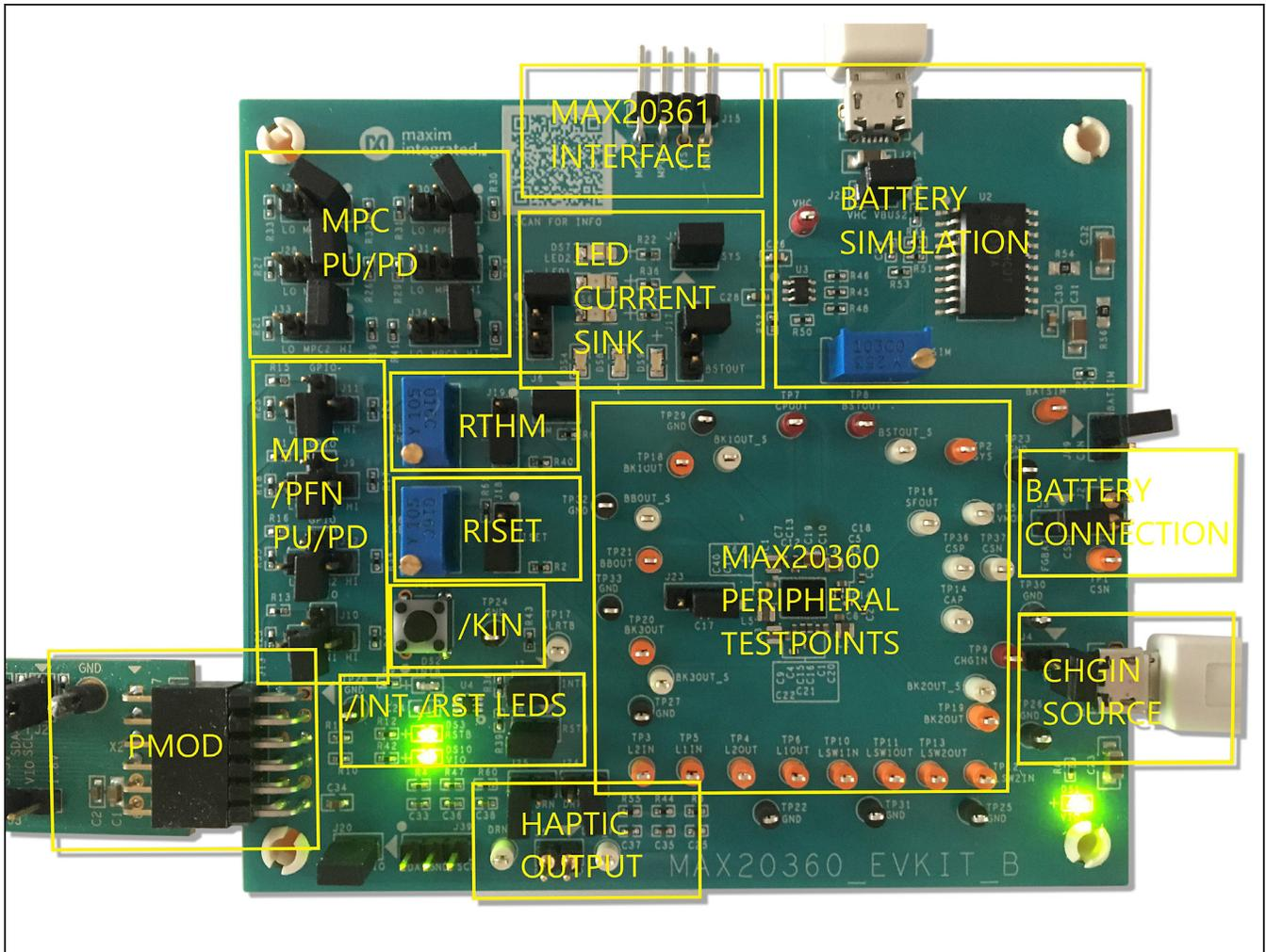
Figure 16. MAX20360 EV Kit Block Annotated Picture
