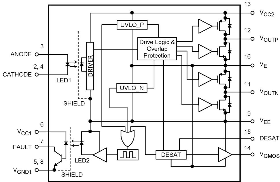
Note: A 10 $\mu$ F bypass capacitor must be connected between pins 9 and 13, and A 1 $\mu$ F bypass capacitor must be connected between pins 13 and 16, and pins 9 and 16.
