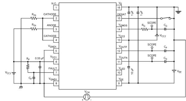
Fig. 13.1.20 CM<sub>L</sub> Refer to V<sub>E</sub> Test Circuit (Gate Output: ON)
