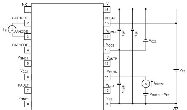
Fig. 13.1.4 I<sub>OUTNL</sub> Test Circuit
