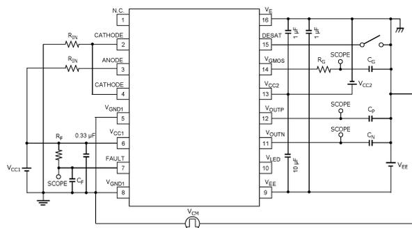
Fig. 13.1.21 CM<sub>H</sub> Refer to V<sub>GND1</sub> Test Circuit (Fault Output: HIGH)
