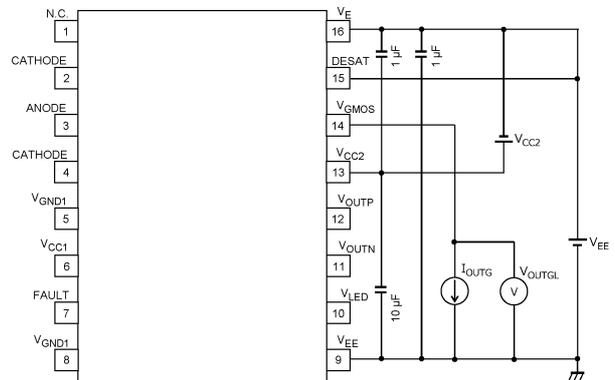
Fig. 13.1.12 V<sub>OUTGL</sub>, R<sub>OUTGL</sub> Test Circuit
