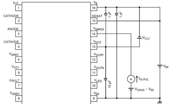
Fig. 13.1.10 I<sub>OUTGL</sub> Test Circuit
