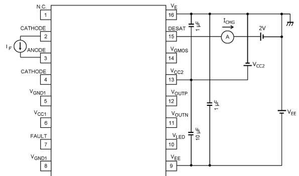
Fig. 13.1.16 I<sub>CHG</sub> Test Circuit
