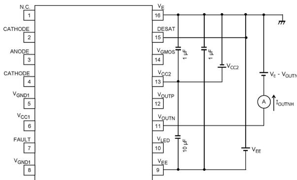
Fig. 13.1.3 I<sub>OUTNH</sub> Test Circuit
