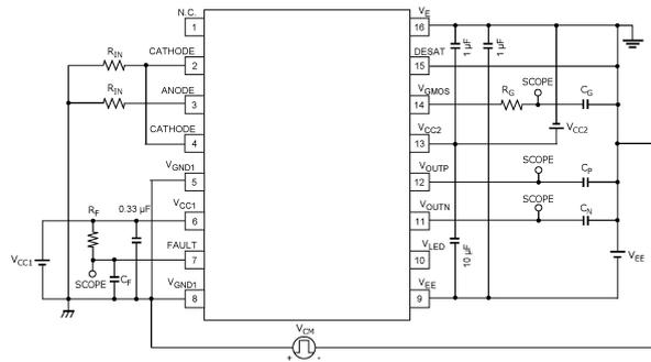
Fig. 13.1.19 CM<sub>H</sub> Refer to V<sub>E</sub> Test Circuit (Gate Output: OFF)
