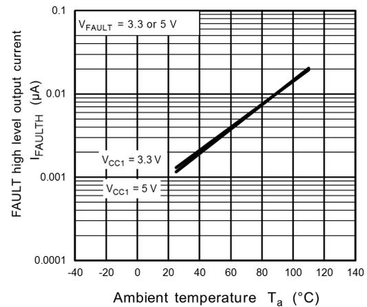
**Fig. 13.3.28**  $I_{FAULTH} - T_a$
