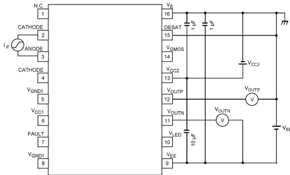
Fig. 13.1.15 I<sub>FHL</sub>, I<sub>FLH</sub> Test Circuit
