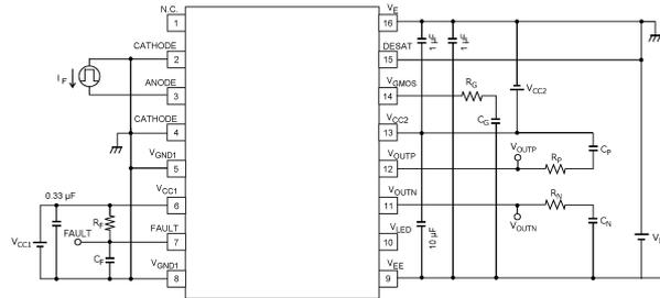
Fig. 13.1.17 t<sub>pLH</sub>, t<sub>pHL</sub>, t<sub>nLH</sub>, t<sub>nHL</sub>, t<sub>DP</sub>, t<sub>DN</sub>, t<sub>PR</sub>, t<sub>PF</sub>, t<sub>NR</sub>, t<sub>NF</sub> Test Circuit
