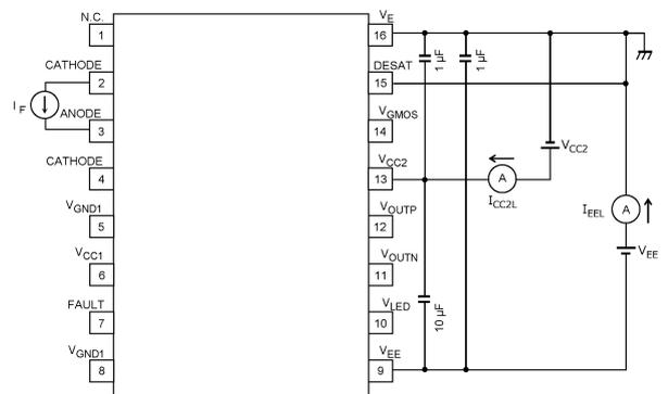
Fig. 13.1.14 I<sub>CC2L</sub>, I<sub>EEL</sub> Test Circuit
