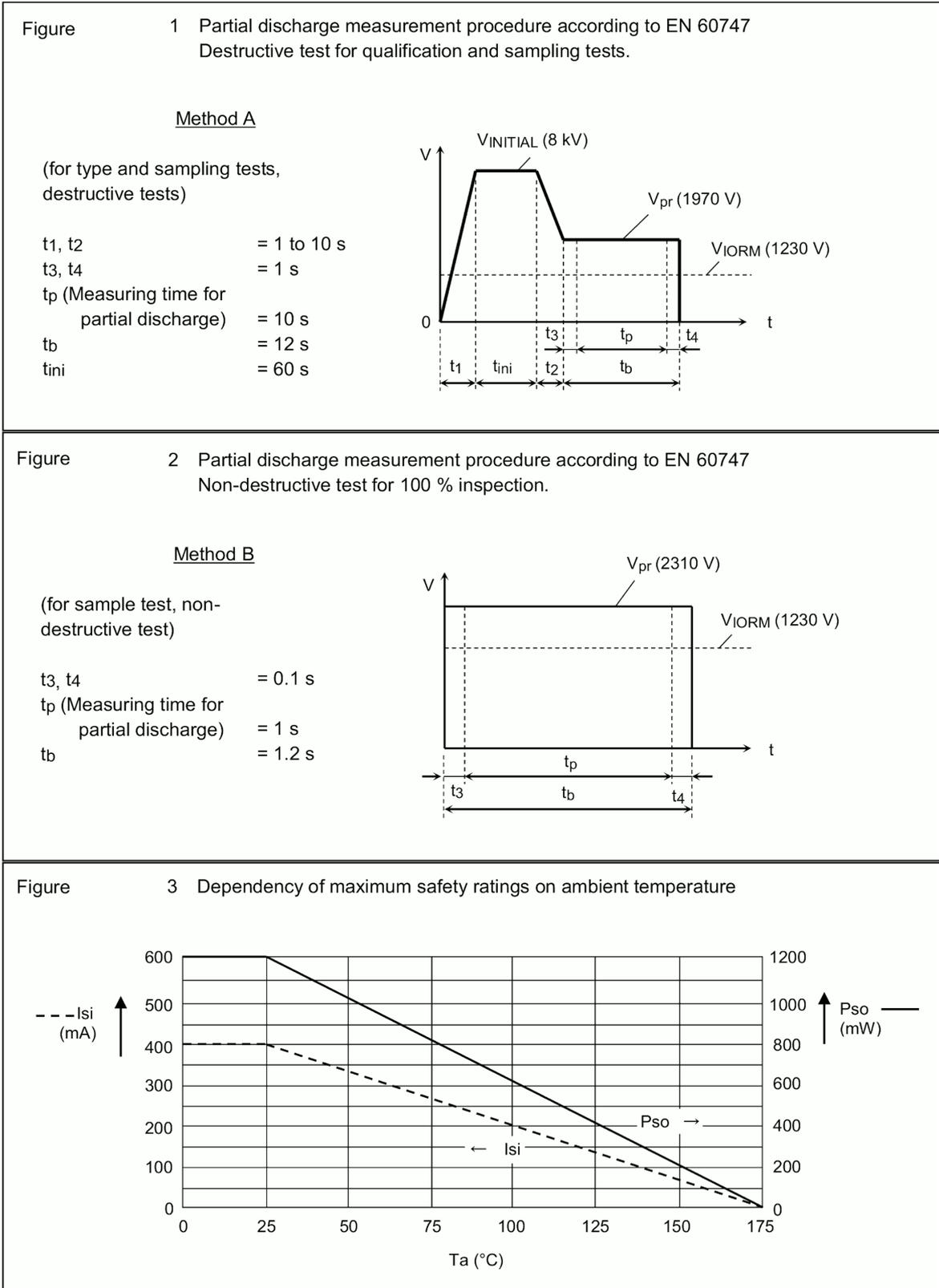
Fig. 17.5 Measurement Procedure
