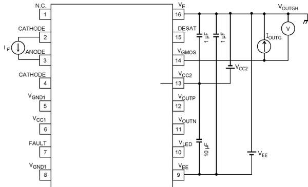
Fig. 13.1.11 V<sub>OUTGH</sub>, R<sub>OUTGH</sub> Test Circuit
