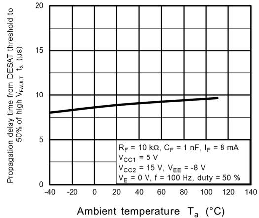
**Fig. 13.3.32  $t_3 - T_a$**
