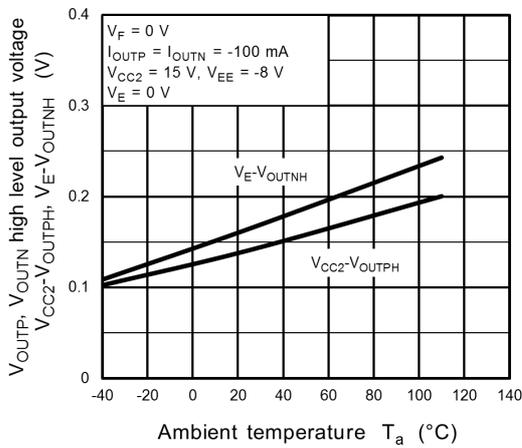
Fig. 13.3.15  $V_{CC2} - V_{OUTPH}, V_E - V_{OUTNH} - T_a$
