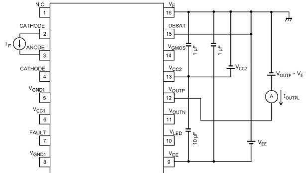
Fig. 13.1.2 I<sub>OUTPL</sub> Test Circuit
