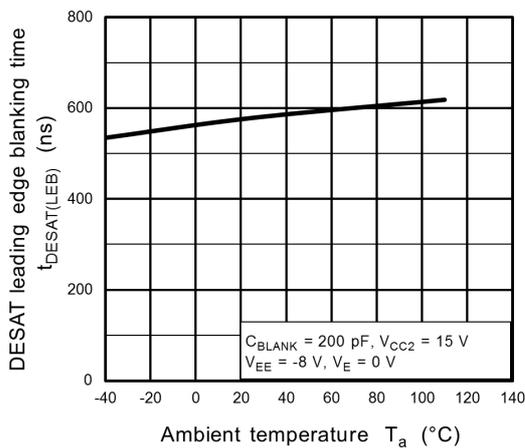
**Fig. 13.3.35  $t_{DESAT(LEB)} - T_a$**
