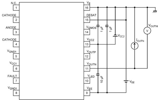
Fig. 13.1.7 V<sub>OUTNH</sub>, R<sub>OUTNH</sub> Test Circuit
