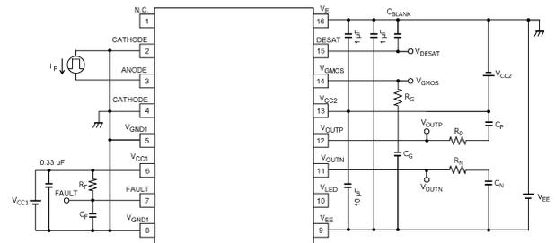
Fig. 13.1.18 t<sub>1</sub>, t<sub>2</sub>, t<sub>3</sub>, t<sub>4</sub>, t<sub>MUTE</sub> Test Circuit
