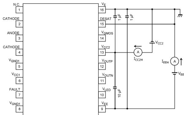
Fig. 13.1.13 I<sub>CC2H</sub>, I<sub>EEH</sub> Test Circuit
