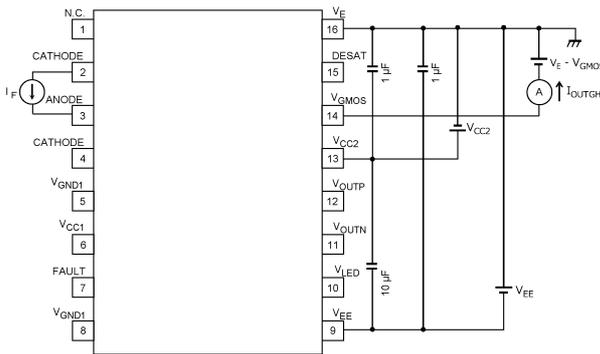
Fig. 13.1.9 I<sub>OUTGH</sub> Test Circuit
