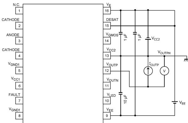
Fig. 13.1.5 V<sub>OUTPH</sub>, R<sub>OUTPH</sub> Test Circuit
