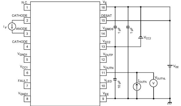
Fig. 13.1.8 V<sub>OUTNL</sub>, R<sub>OUTNL</sub> Test Circuit
