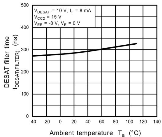
**Fig. 13.3.36  $t_{DESAT(FILTER)} - T_a$**
