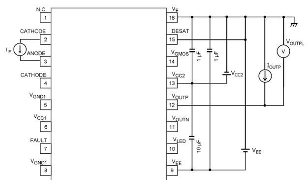
Fig. 13.1.6 V<sub>OUTPL</sub>, R<sub>OUTPL</sub> Test Circuit
