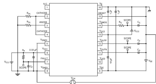
Fig. 13.1.22 CM<sub>L</sub> Refer to V<sub>GND1</sub> Test Circuit (Fault Output: LOW)
