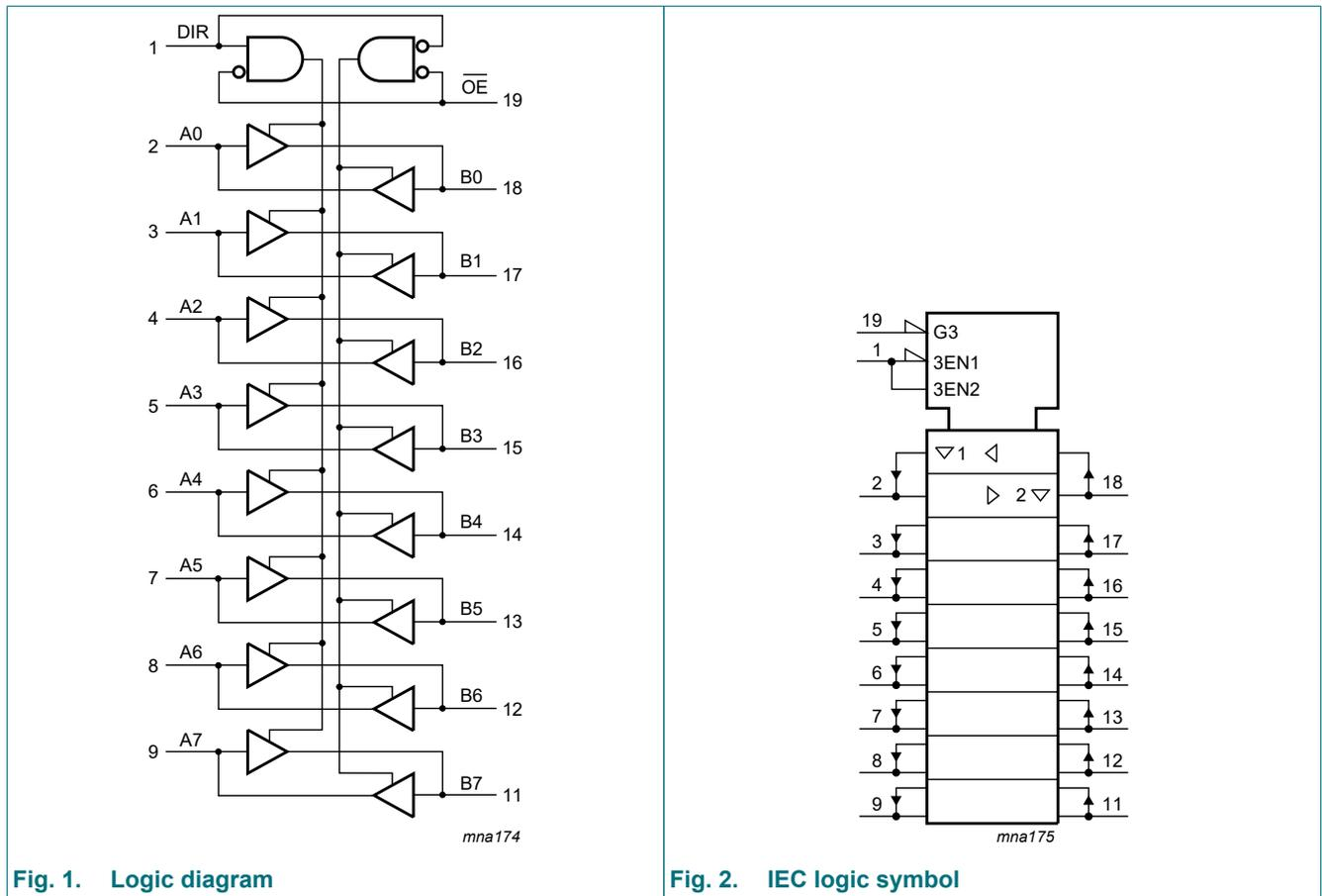
Fig. 1. Logic diagram
