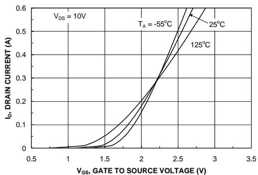
Figure 5. Transfer Characteristics.
