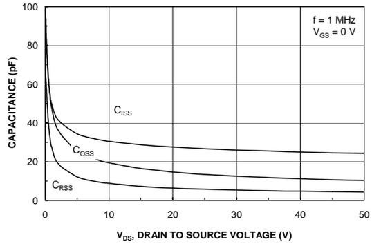
Figure 8. Capacitance Characteristics.
