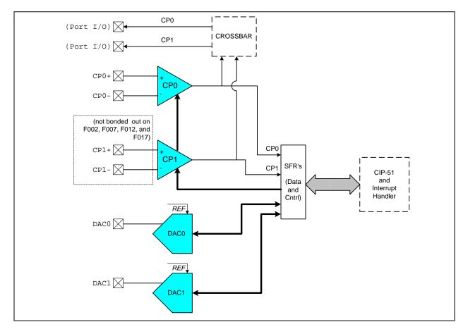
Figure 1.11. Comparator and DAC Diagram
