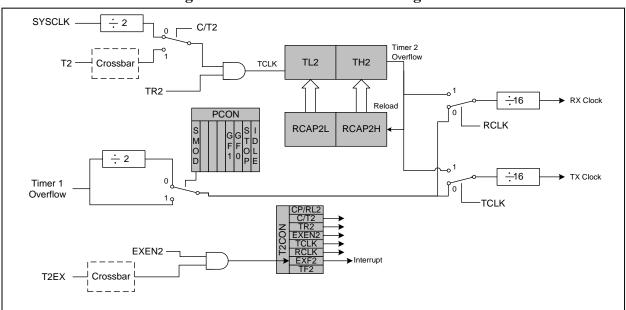
Figure 19.13. T2 Mode 2 Block Diagram
