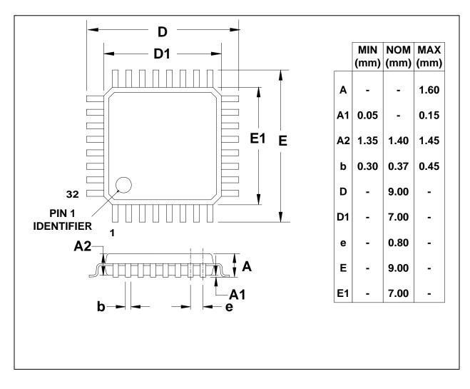
Figure 4.6. LQFP-32 Package Drawing
