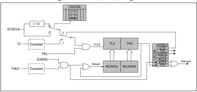
Figure 19.12. T2 Mode 1 Block Diagram
