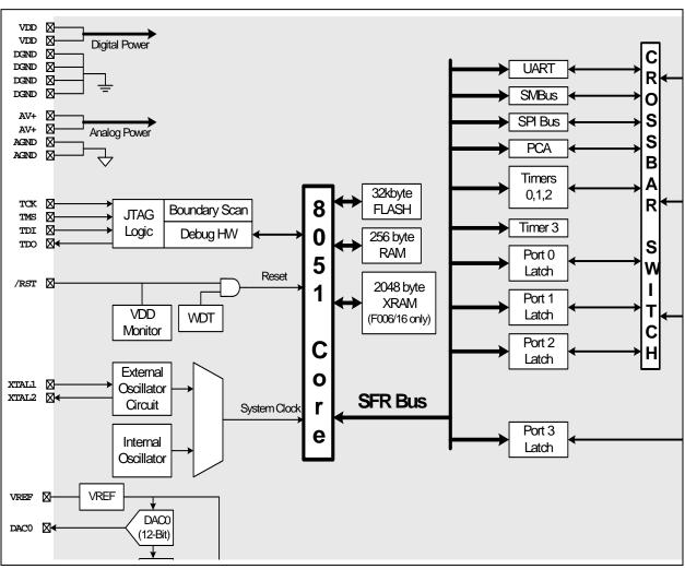
Figure 1.2. C8051F001/06/11/16 Block Diagram
