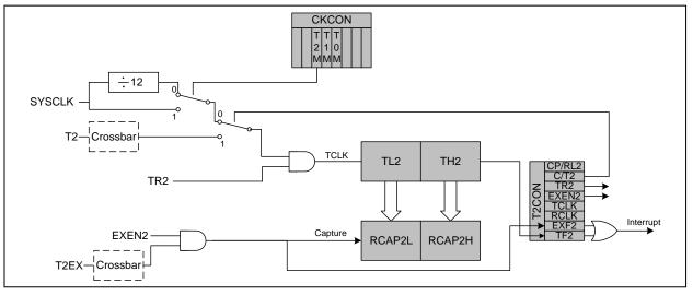
Figure 19.11. T2 Mode 0 Block Diagram
