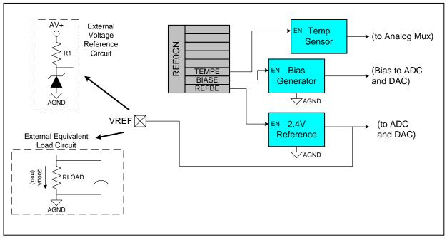
Figure 9.1. Voltage Reference Functional Block Diagram
