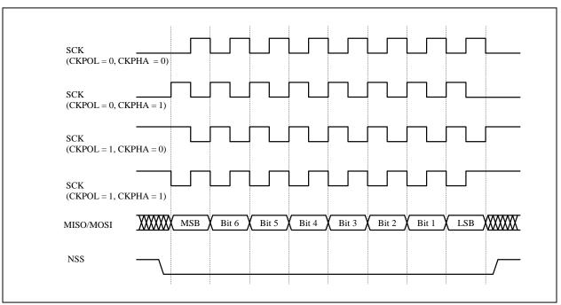
Figure 17.4. Data/Clock Timing Diagram
