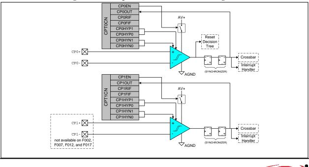
Figure 8.1. Comparator Functional Block Diagram
