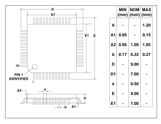
Figure 4.4. TQFP-48 Package Drawing
