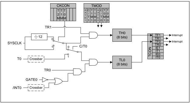
Figure 19.3. T0 Mode 3 Block Diagram
