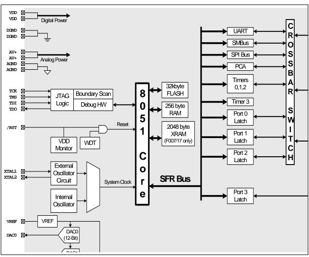
Figure 1.3. C8051F002/07/12/17 Block Diagram
