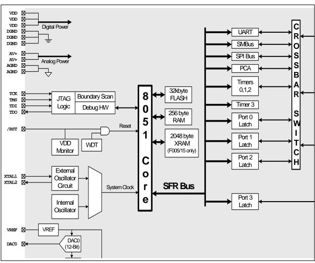
Figure 1.1. C8051F000/05/10/15 Block Diagram
