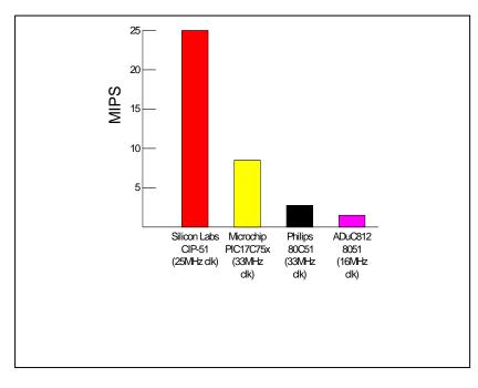
Figure 1.4. Comparison of Peak MCU Execution Speeds
