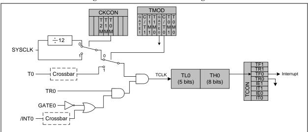
Figure 19.1. T0 Mode 0 Block Diagram
