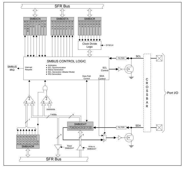
Figure 16.1. SMBus Block Diagram
