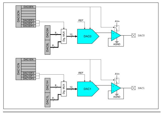
Figure 7.1. DAC Functional Block Diagram
