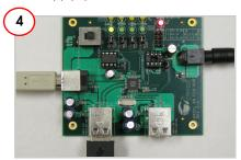
Connect a USB device to any of the four downstream ports. Use jumpers J7 to J10 in position 2-3 to enable the corresponding port status LEDs. The red LED glowing indicates that the hub is not in Suspend mode. The green LED glowing indicates that the respective downstream port is enabled.
