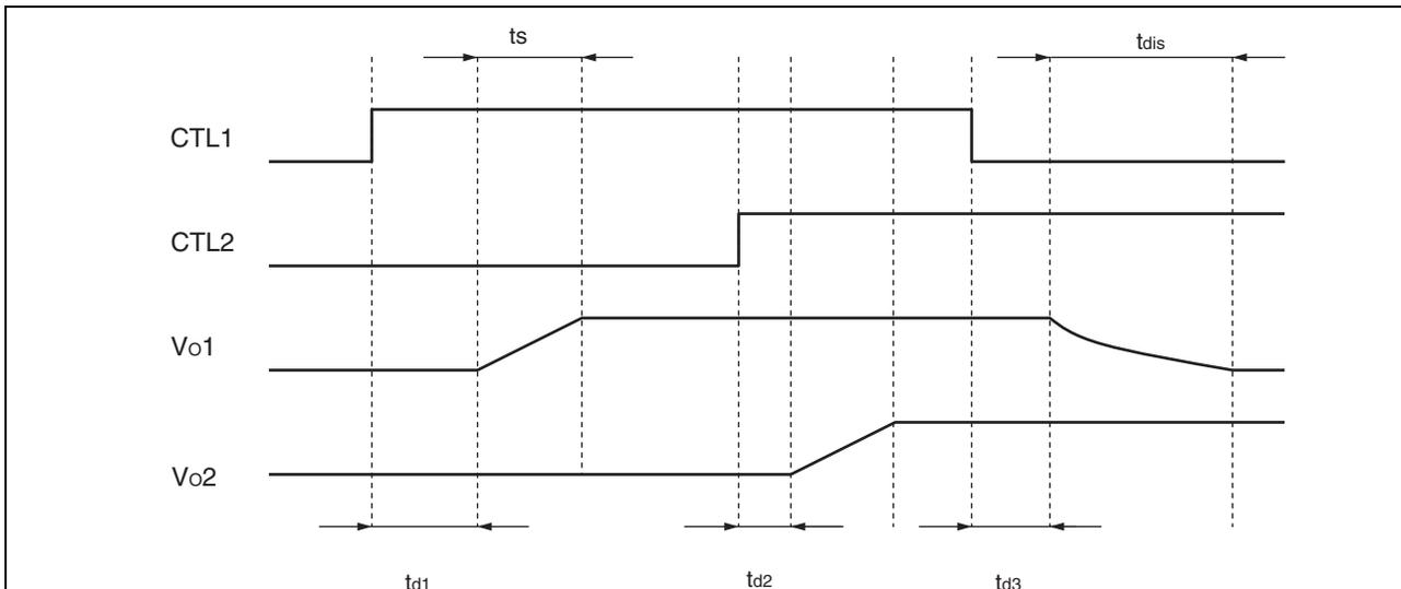
■ Simultaneous operation of plural channels
