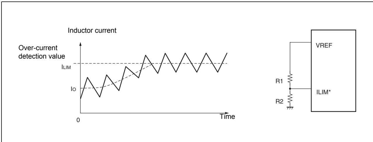
\* If the over current detection function is not used, connect the  $I_{LIM}$  pin ( $I_{LIM1}$  and  $I_{LIM2}$ ) to the  $V_{REF}$  pin.
