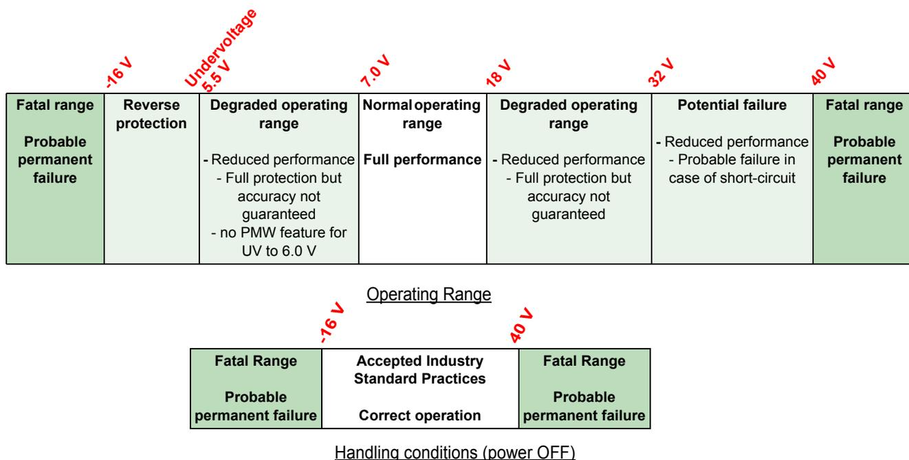
**Figure 4. Ratings vs. operating requirements (VBAT pin)**
