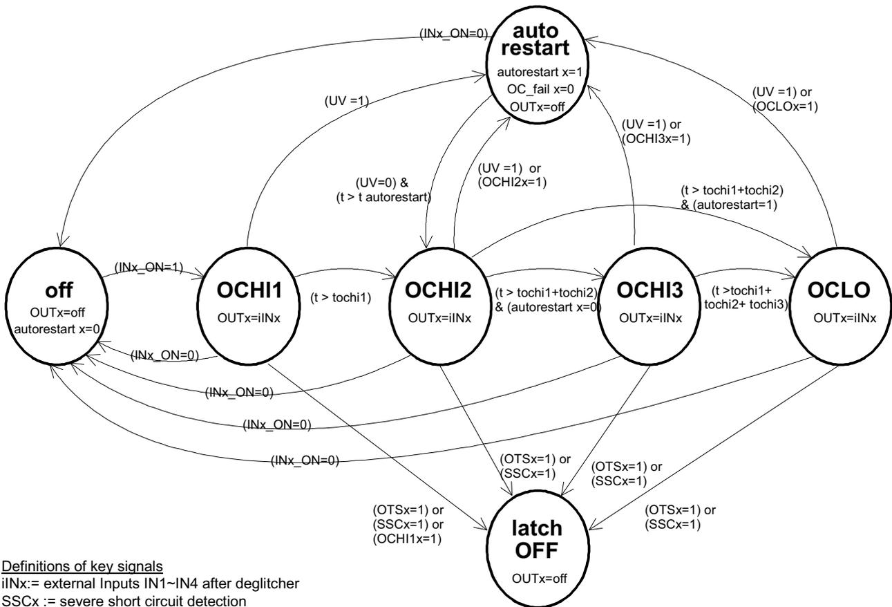
**Figure 14. Output control diagram in fail mode**
