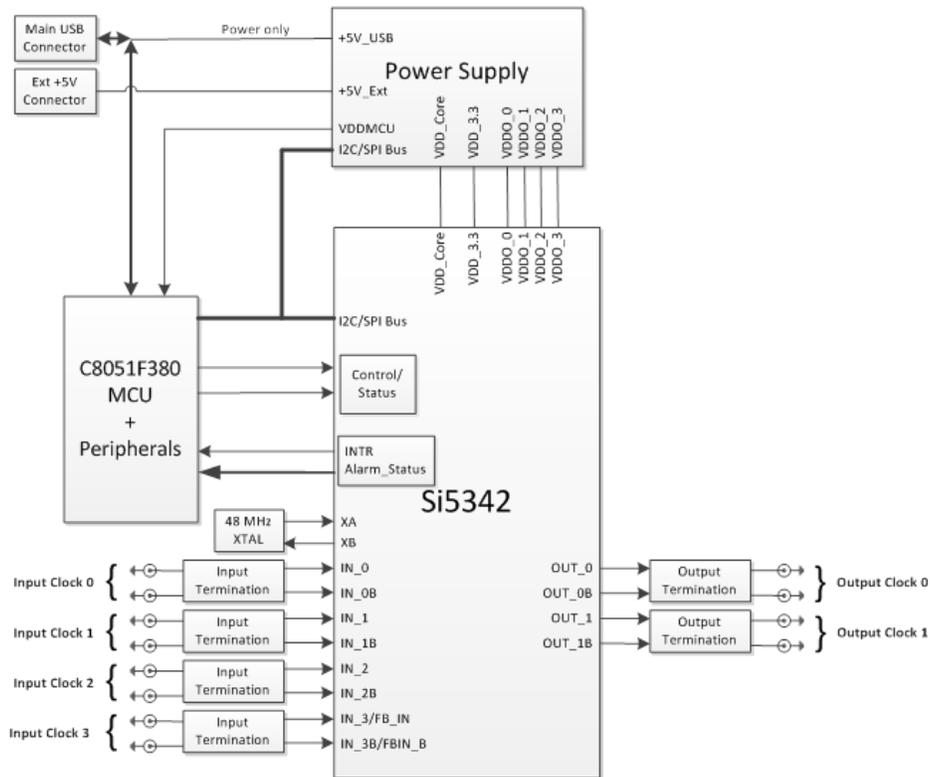
Figure 2. Si5342-EVB Functional Block Diagram
