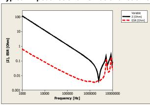
V<sub>DC</sub> = 0 V, V<sub>AC</sub> = 0.5 V<sub>RMS</sub>, T<sub>device</sub> = +25 °C
