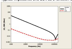
$V_{DC} = 0 V$ ,  $V_{AC} = 0.5 V_{RMS}$ ,  $T_{device} = +25 °C$
