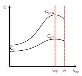
Initial capacitance  $C_0$ : Is the value at the origin of the hysteresis without any applied direct
