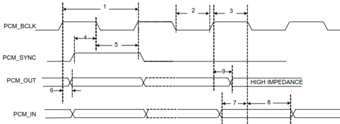
Figure 3: PCM timing diagram (Short-Frame Sync, Slave Mode)
