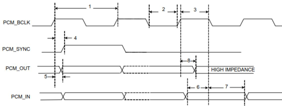
Figure 2: PCM timing diagram (Short-Frame Sync, Master Mode)
