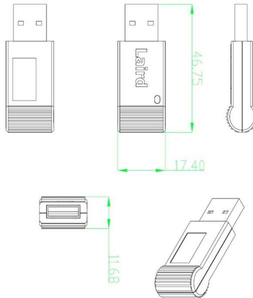
Figure 16: BT851 USB dongle, containing embedded BT850-SA
