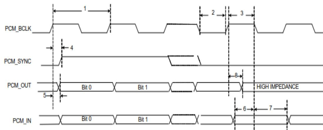
Figure 4: PCM timing diagram (Long-Frame Sync, Master Mode)
