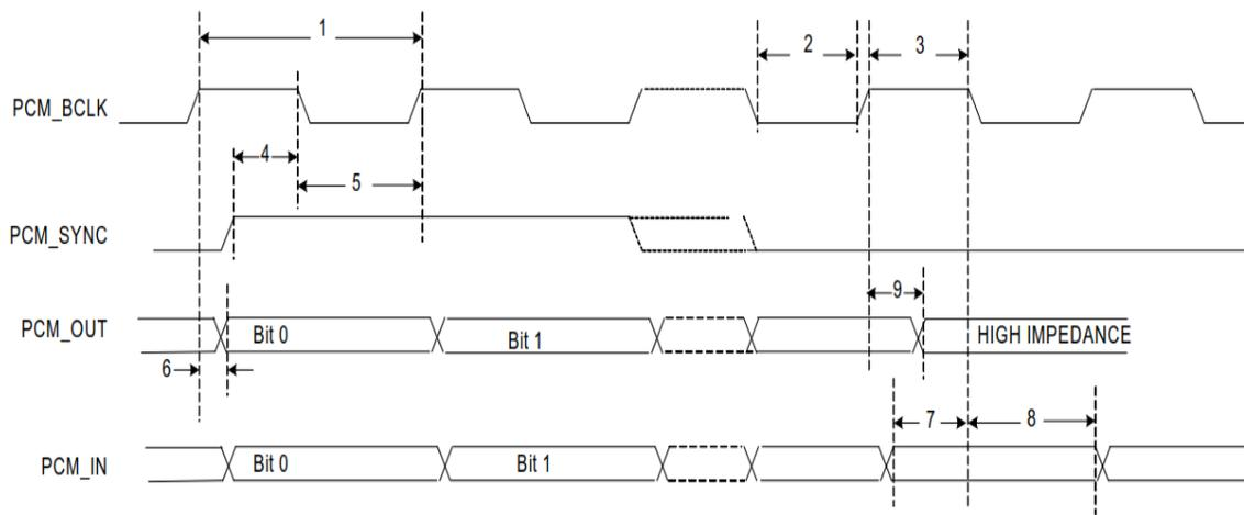
**Figure 5: PCM timing diagram (Long-Frame Sync, Slave Mode)**
