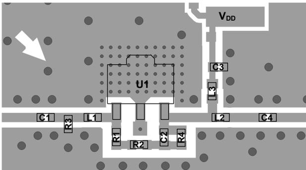
The bias current can be adjusted to support lower noise figure and lower power consumption by removing external bias resistor R4 and replacing R3 as detailed below.
