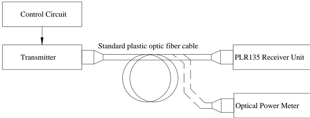
\*Fig.2 Measuring Method of Dissipation Current
