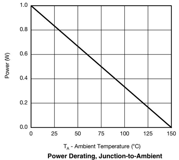
\* The power dissipation  $P_D$  is based on  $T_{J(max)} = 150\text{ }^\circ\text{C}$ , using junction-to-case thermal resistance, and is more useful in settling the upper dissipation limit for cases where additional heatsinking is used. It is used to determine the current rating, when this rating falls below the package limit.
