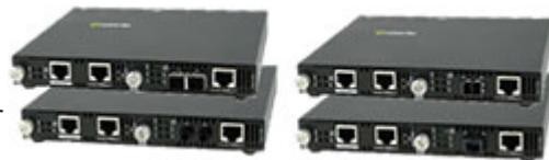
Perle's advanced line of **Managed Gigabit Media Converters**, provides transparent and reliable **Gigabit Ethernet to fiber connections**. While providing an economical means of extending your existing copper based network connection, these media converters are SNMP manageable to enable complete control and status viewing of your fiber links.
