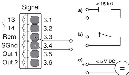
To switch the power supply back on, select one of the following external circuits between signal terminal blocks Rem and SGnd. Power transmission inside the device is activated again. As usual, the energy for supplying the loads is available at the DC output terminal blocks.
