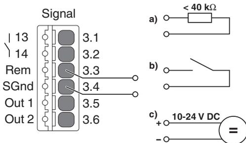
When using a PLC output, select the following external circuit version to switch the power supply to SLEEP MODE.
