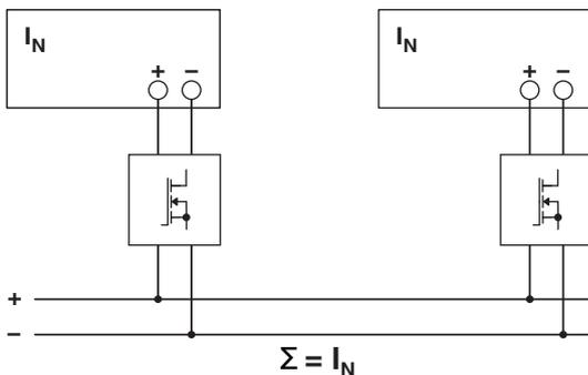
Certain specifications apply in redundancy operation with regard to the configuration of the keepout areas. In redundancy operation, the power supplies are operated with maximum half the nominal power. The keepout areas are therefore reduced.
