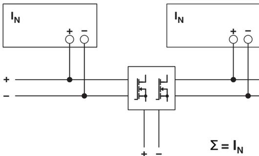
Figure 44 Schematic diagram, redundant operation with QUINT S-ORING
