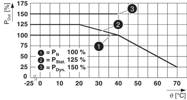
16.4.6 Rotated mounting position 270° X-axis
