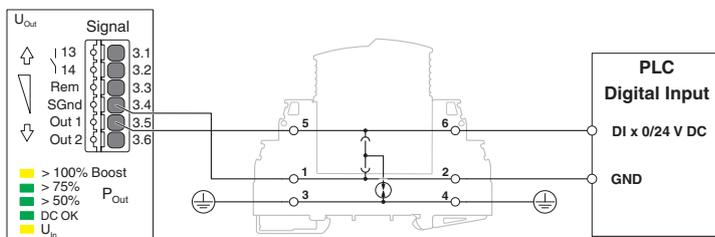
Figure 40 Schematic diagram, signal wiring with relay module
