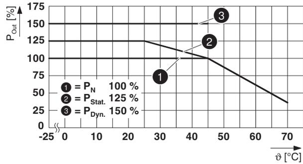
16.4.5 Rotated mounting position 90° X-axis
