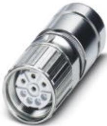
Cable connector, straight short, Screw locking, M23, Number of positions: 4+3+PE, Type of contact: Socket, Crimp connection, Shielded: Yes, Cable cross section: 7.5 mm...9 mm
