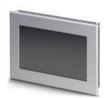
Rugged-Touch panel with 17.8 cm/7" TFT-display (Analog resistive (GFG)), 800 x 480 pixel(s) (WVGA), 65536 colors, Arm<sup>®</sup> Cortex<sup>®</sup>-A8, 1000 MHz, 2x USB host 2.0, 1 x Ethernet (10/100 Mbps), RJ45, Windows<sup>®</sup> Embedded Compact 7 and user software: Visu+. (bus system: without)
