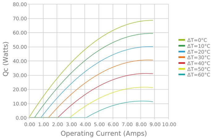
Heat Pumped at Cold Side
