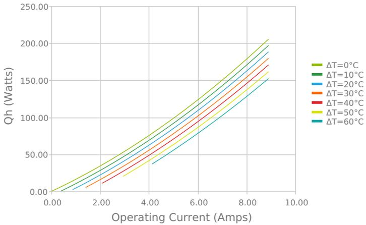
Total Heat Dissipated at Hot Side (Qh=Qc+Pin)
