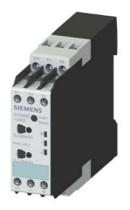
Insulation monitoring relay for ungrounded (IT) supply systems up to 250 V AC, 15-400 Hz and up to 300 V DC Measuring range 1-100 kohm Supply voltage 24-240 V AC/DC 22.5 mm, 1 change-over contact screw terminal
