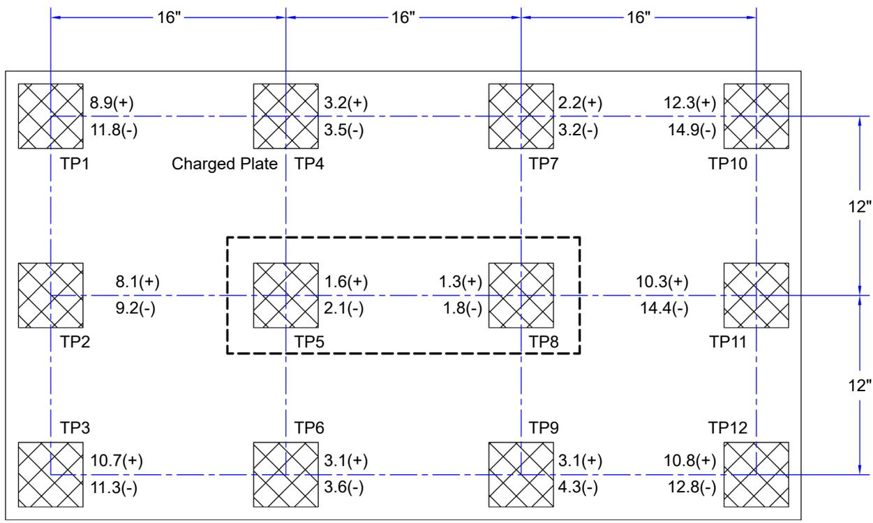
Figure 16. 60640, 60467 Neutralization (Discharge) Times at 220VAC, 50Hz input
