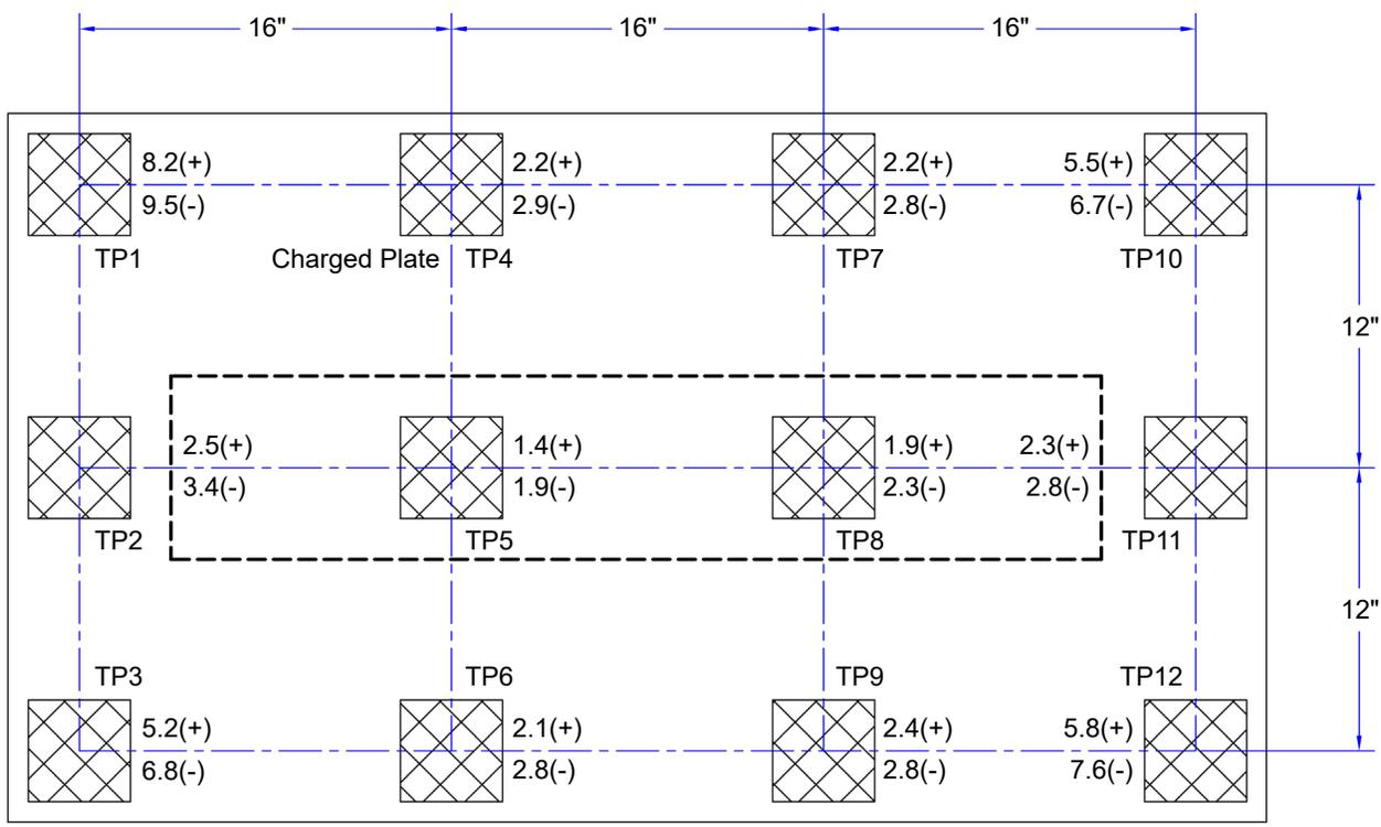
Figure 12. 60473, 60468 Neutralization (Discharge) Times at 120VAC, 60Hz input
