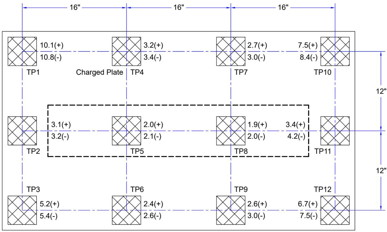
Figure 13. 60473, 60468 Neutralization (Discharge) Times at 220VAC, 50Hz input
