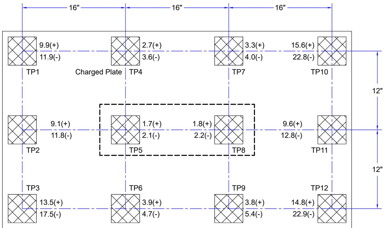
Figure 14. 60640, 60467 Neutralization (Discharge) Times at 100VAC, 50Hz input
