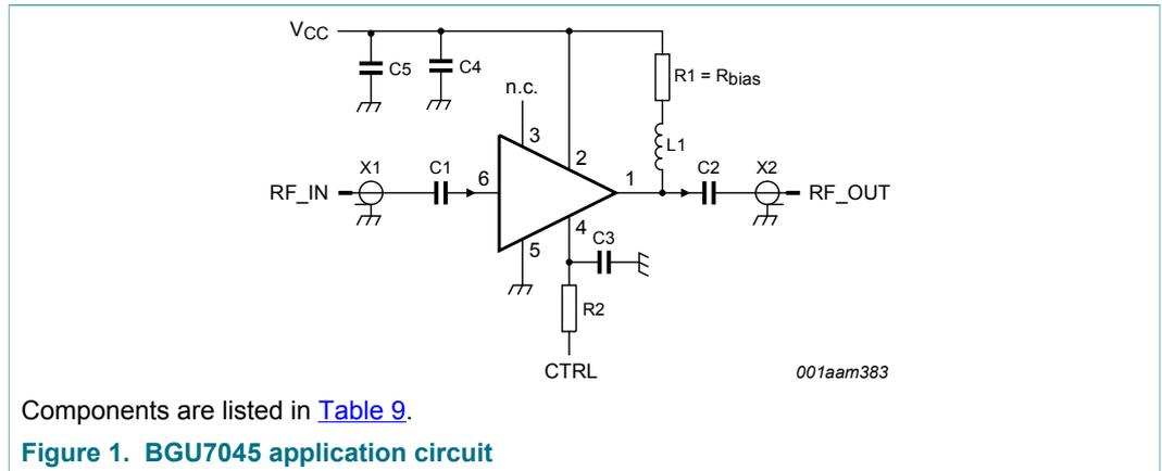
All control and supply lines must be decoupled properly. The decoupling capacitors must be placed as close to the device as possible.
