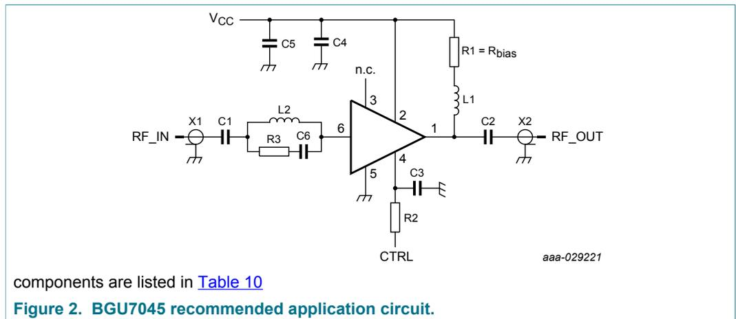
(Values can be changed depending on the PCB routing) Keep the components (L2, R3, C6) next to the BGU7045 RF input pin.
