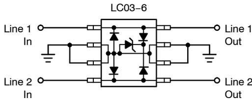
**Figure 5. Configuration for Differential and Common Mode Protection**
