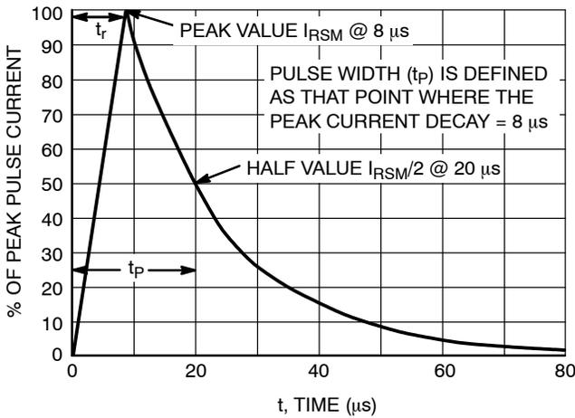
Figure 3. 8 x 20  $\mu\text{s}$  Pulse Waveform
