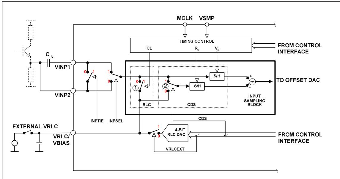
Figure 4 Reset Level Clamping and CDS Circuitry
