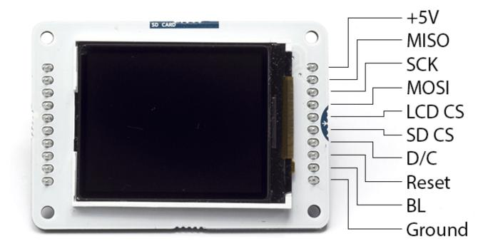
The screen is 1.77" diagonal, with 160 x 128 pixel resolution. The TFT library interfaces with the screen's controller through SPI when using the TFT library. Refer to the screen's data sheet for complete details.
