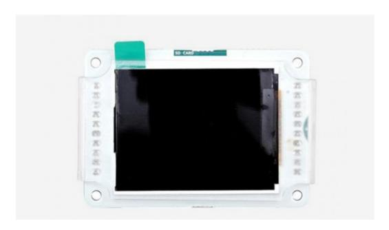
Use this small LCD screen with Arduino Robot, Esplora, or on breadboard.
