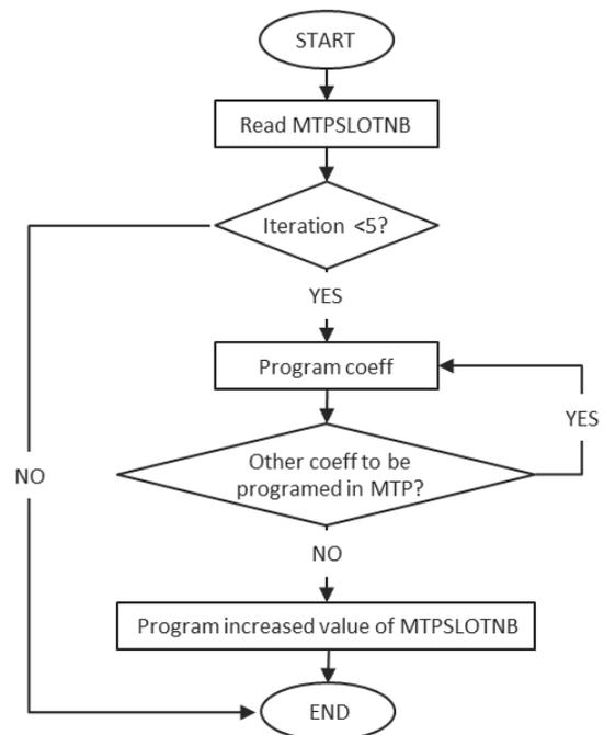
Figure 26: Procedure to program new calibration parameters
