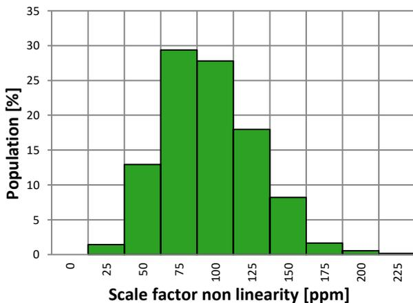
Figure 4: Scale Factor non linearity distribution (room temperature)
