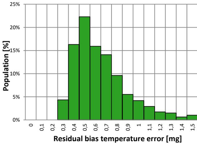
Figure 2: Residual bias temperature error distribution, absolute value
