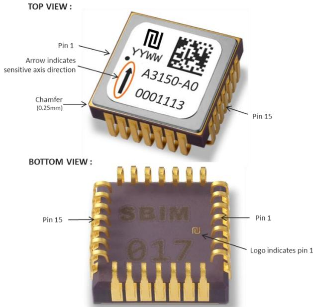
Figure 12: How to locate Pin 1 and Sensitive Axis
