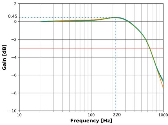
Figure 9: Frequency response (3 samples at room temperature)
