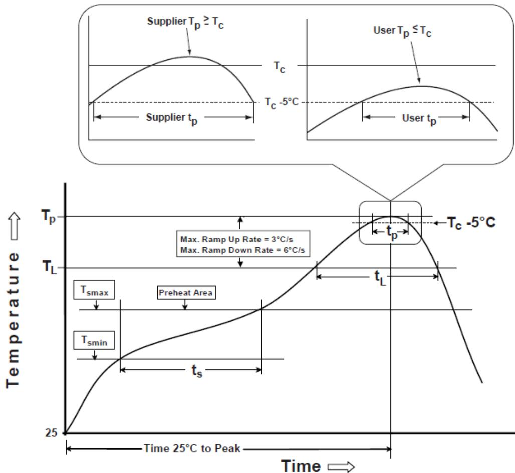
Figure 16: Reflow Profile, according to IPC/JEDEC J-STD-020D.1
