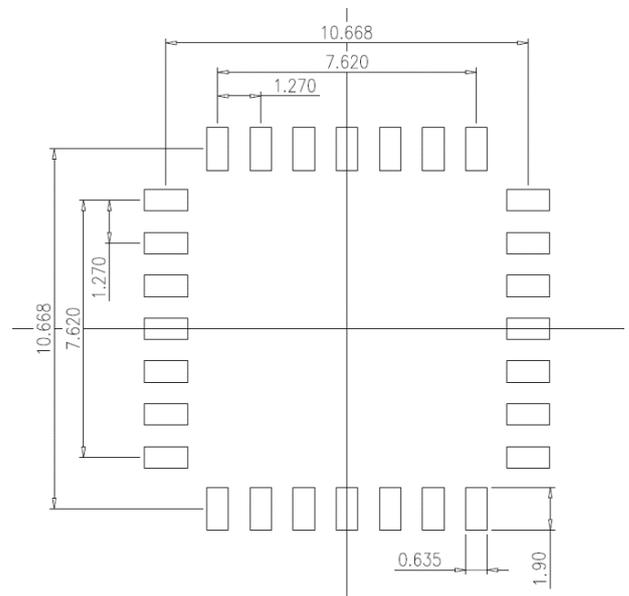
Figure 15: Recommended Pad Layout (dimensions in mm)
