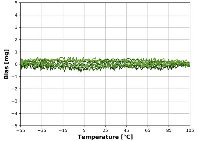
Figure 5: Residual bias temperature error (5 samples)
