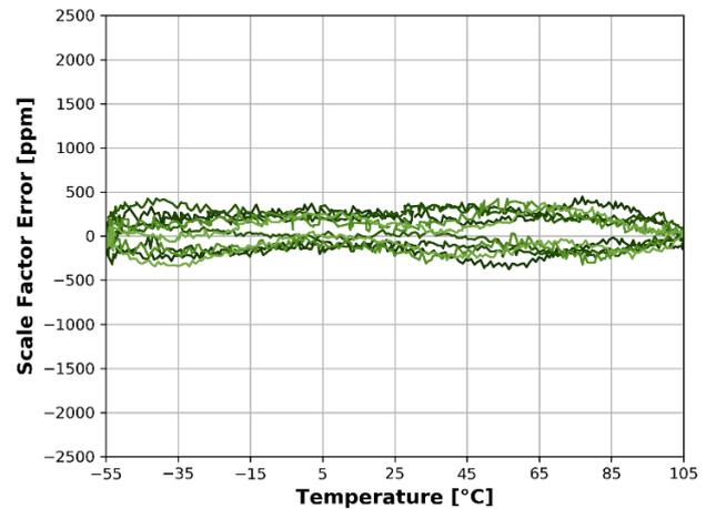
Figure 6: Residual scale factor temperature error (5 samples)
