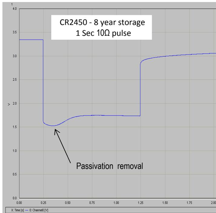
The passivation layer due to long term storage can contribute to a slightly higher initial internal resistance and subsequently an increased voltage drop when the battery is first put into use. Once a load is placed on the battery, the passivation layer will become thinner, and internal resistance typically returns to normal.
