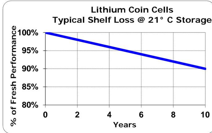
When stored at normal room temperature and humidity, Lithium coin cells will lose approximately 1% of their capacity per year due to ingress and egress of vapors through the seal. When lithium coin cells have been stored for years in a sealed package, the smell of DME (1, 2-Dimethoxy Ethane) is sometimes noticeable when the packaging is first opened due to egress through the seal. The DME vapor has an ether like odor but there is not a safety concern.
