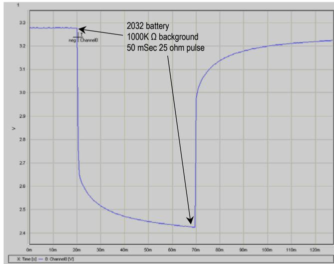
In low drain continuous applications (i.e. watch) the battery IR may not be a critical factor. However, in high pulse applications (i.e. wireless sensors), the battery IR can significantly impact runtime due to voltage drop. The battery IR will typically increase during discharge due to the impact of the reaction by-products on the battery chemistry.
