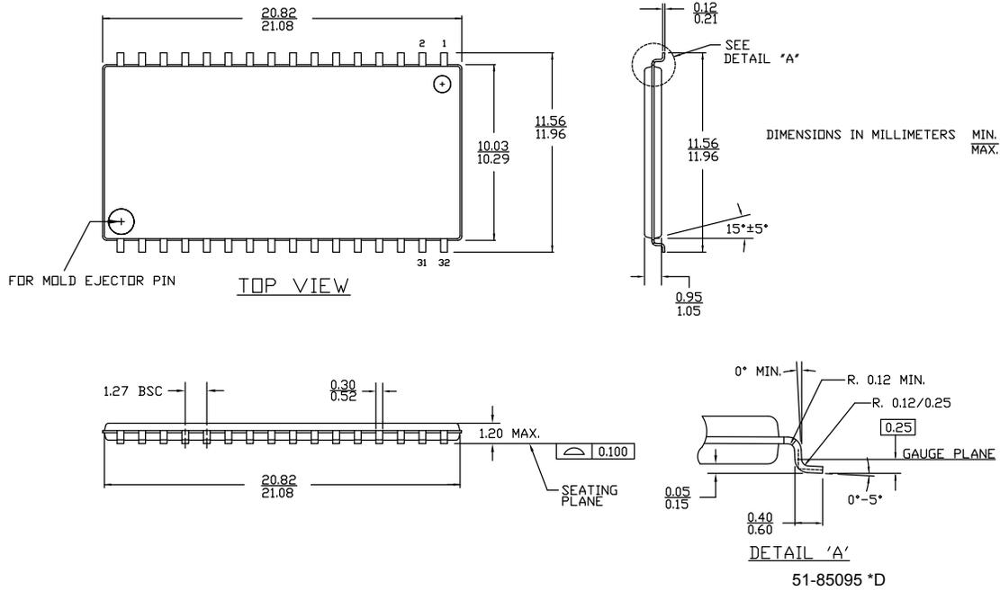
Figure 10. 32-pin SOIC (450 Mils) S32.45/SZ32.45 Package Outline, 51-85081
