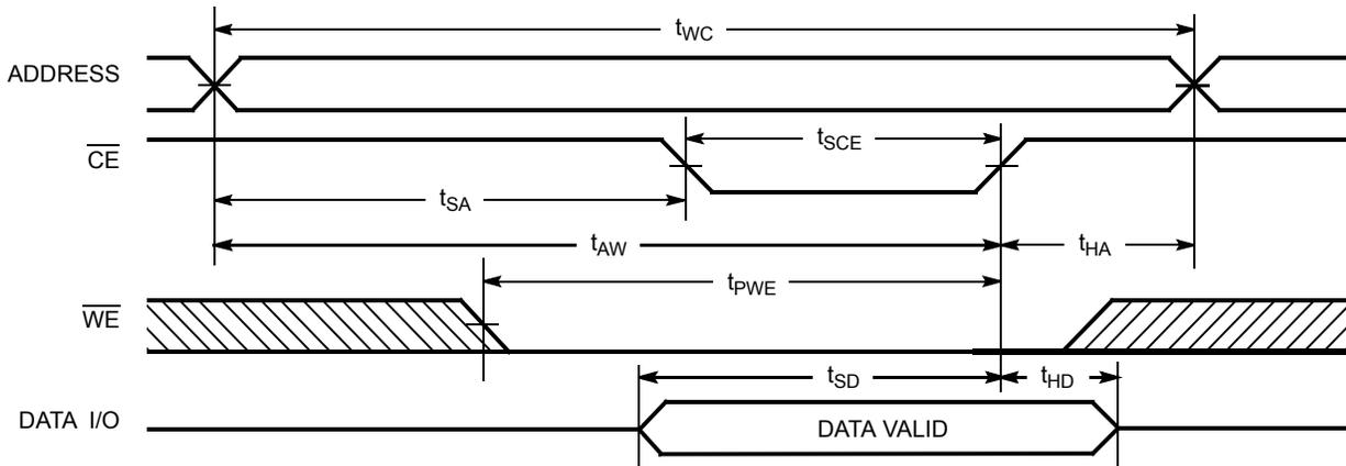
**Figure 8. Write Cycle No. 3 ( $\overline{\text{WE}}$  Controlled,  $\overline{\text{OE}}$  LOW)** [27, 28]
