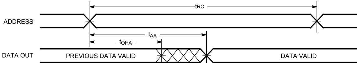
Figure 5. Read Cycle No. 2 ( $\overline{OE}$  Controlled) [21, 22]
