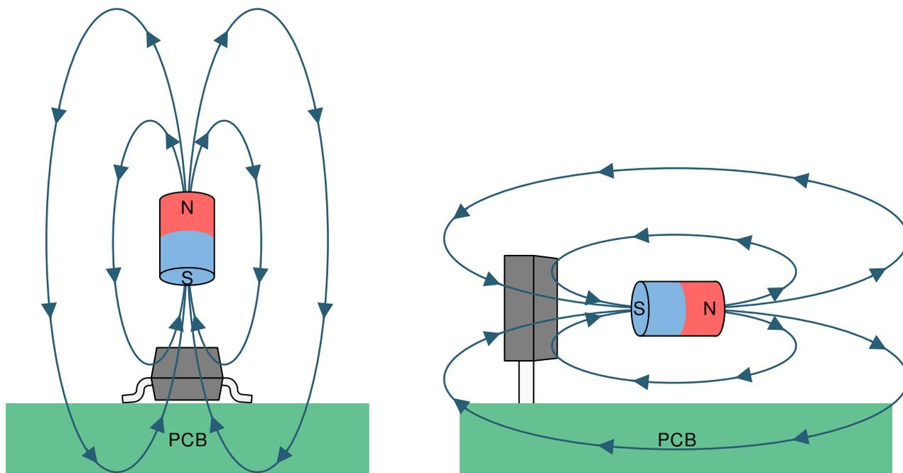
Figure 28. The Flux Direction for Positive B
