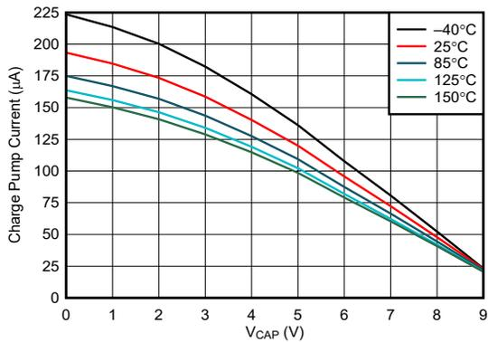
**Figure 6-5. Charge Pump V-I Characteristics at V<sub>SOURCE</sub> = 3.2 V**
