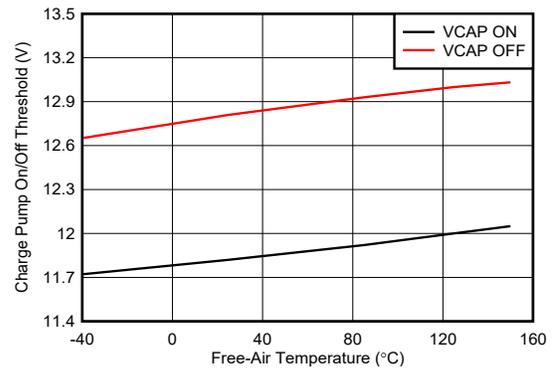
Figure 6-8. Charge Pump ON/OFF Threshold vs Temperature
