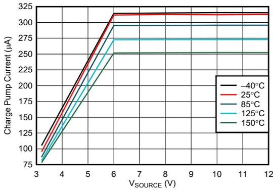
**Figure 6-3. Charge Pump Current vs Supply Voltage at V<sub>CAP</sub> = 6 V**
