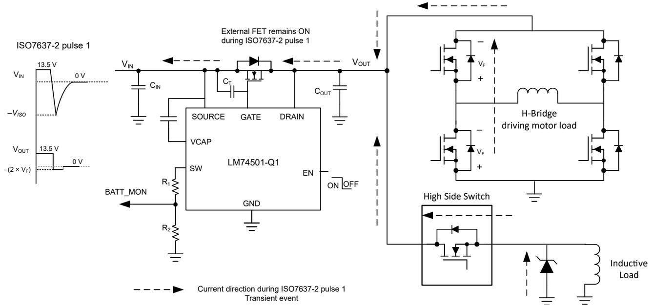
Figure 8-3. Typical Application Scenario During ISO7637-2 Pulse 1 Events
