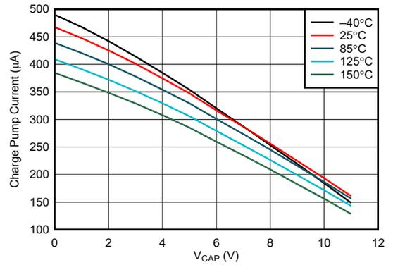
**Figure 6-4. Charge Pump V-I Characteristics at V<sub>SOURCE</sub> >= 12 V**
