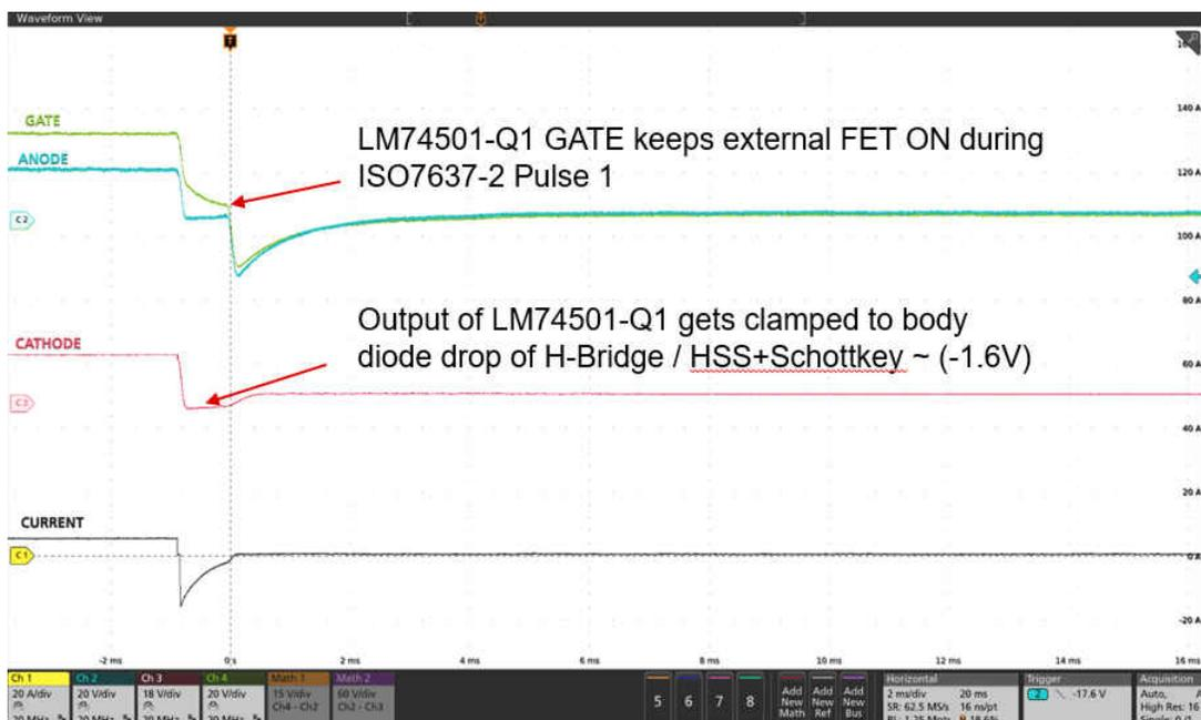
Figure 8-4. TVS Less Operation During ISO7637-2 Pulse 1
