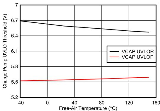
Figure 6-9. Charge Pump UVLO Threshold vs Temperature
