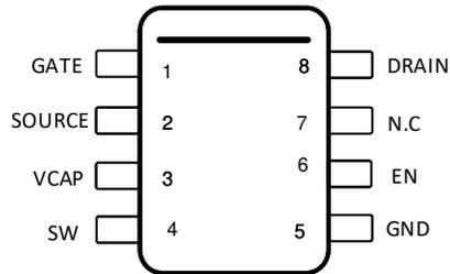
**Figure 5-1. DDF Package 8-Pin SOT-23 (LM74501-Q1 Top View)**
