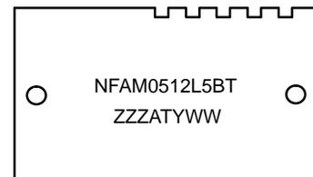
Device marking is on package top side
