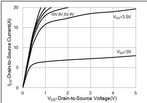
Fig.1 Output Characteristics
