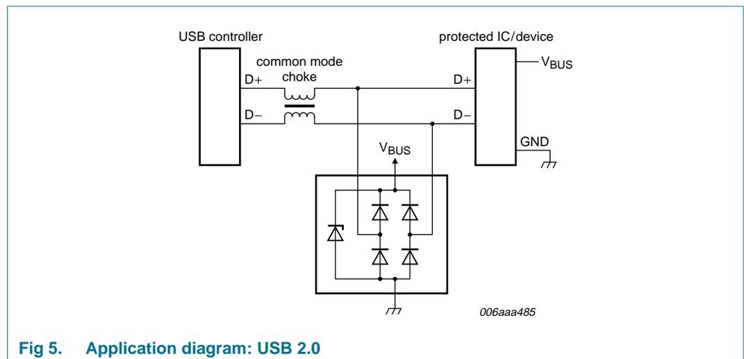
Fig 5. Application diagram: USB 2.0
