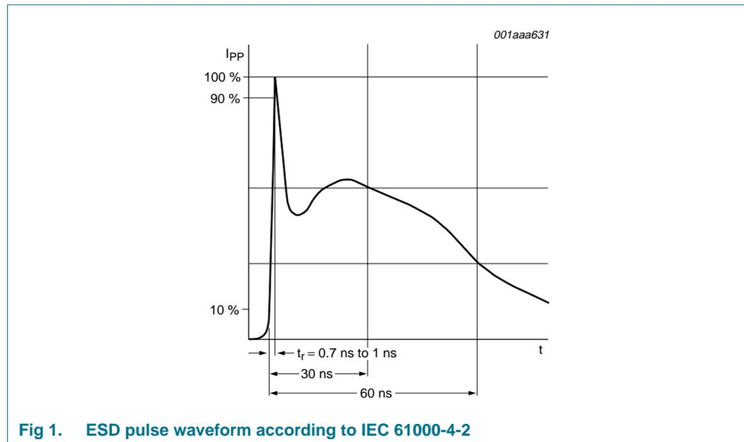
**Fig 1. ESD pulse waveform according to IEC 61000-4-2**
