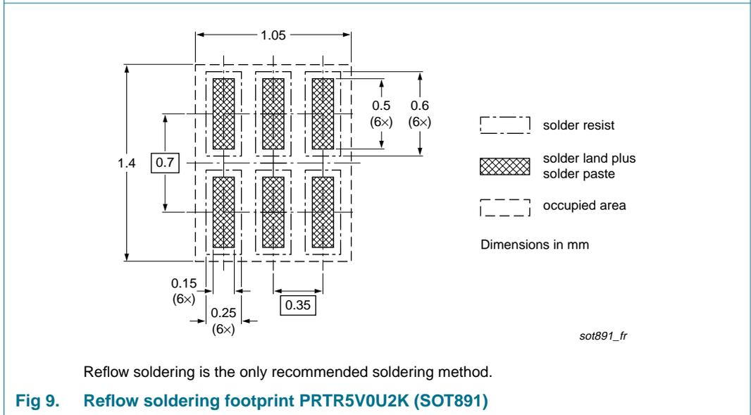
Reflow soldering is the only recommended soldering method.
