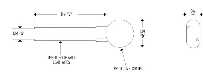
RESISTANCE @  $+25^{\circ}C = 12~\Omega \pm 20\%$  MAXIMUM STEADY STATE CURRENT = 1 AMP RESISTANCE @ MAXIMUM CURRENT = 1.190  $\Omega$  NOMINAL
