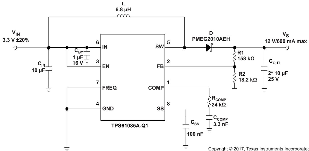
**Figure 14. Typical Application, 3.3 V to 12 V ( $f_{sw} = 650$  kHz)**
