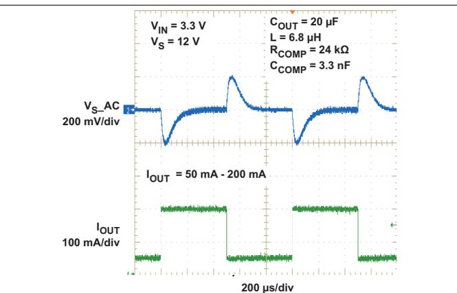
Figure 12. Load Transient Response Low Frequency (650 kHz)
