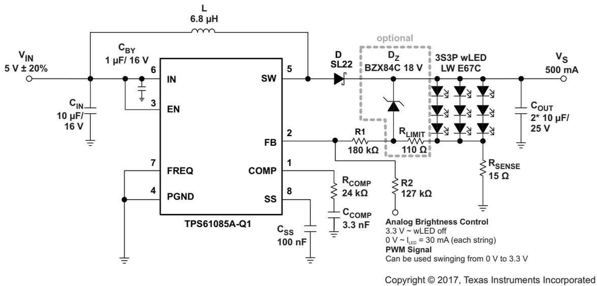
Figure 21. Simple Application (3.3-V Input,  $f_{sw} = 650$  kHz) For wLED Supply (3S3P) With Adjustable Brightness Control Using an Analog Signal on the Feedback Pin (With Optional Clamping Zener Diode)
