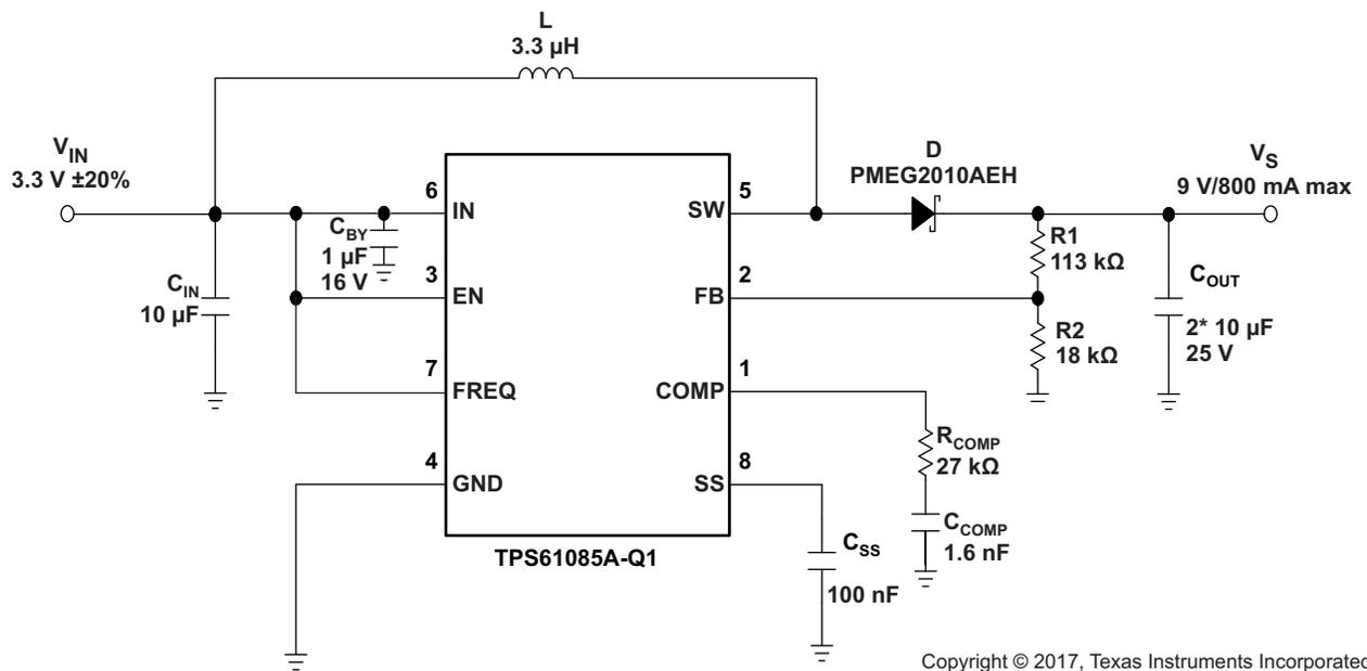
**Figure 15. Typical Application, 3.3 V to 9 V ( $f_{sw} = 1.2$  MHz)**
