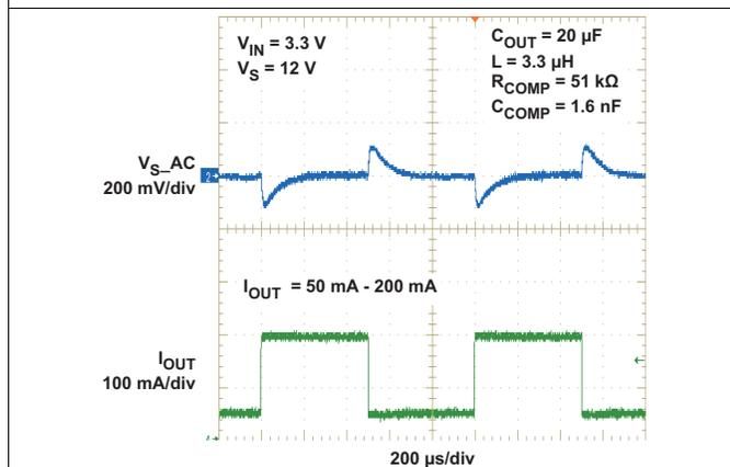
Figure 11. Load Transient Response High Frequency (1.2 MHz)
