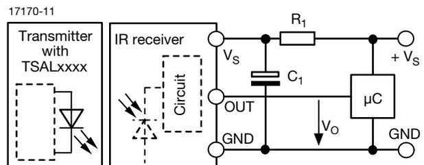
R<sub>1</sub> and C<sub>1</sub> recommended to reduce supply ripple for V<sub>S</sub> < 2.8 V
