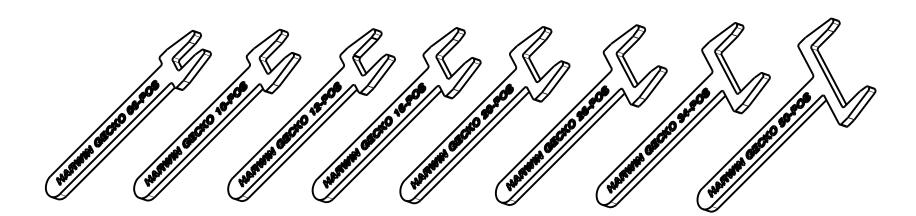
I. TOOLS TO BE USED FOR DELATCHING G125-SERIES CONNECTORS.
