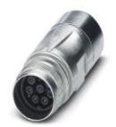
Coupler connector, straight, for standard and SPEEDCON interlock, M17, number of positions: 5+3+PE, type of contact: Socket, Crimp connection, shielded: yes, cable diameter range: 3.5 mm ... 5.5 mm
