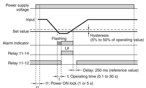
**Note:** The power ON lock prevents unnecessary alarms from being generated during the instable period when the power is first turned on. There is no relay output during timer operation.
