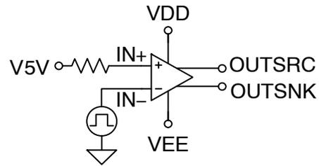
Figure 31. Inverting input configuration
