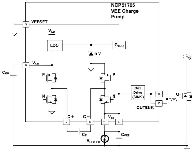
**Figure 34. Supplying VEE with negative external voltage bias**
