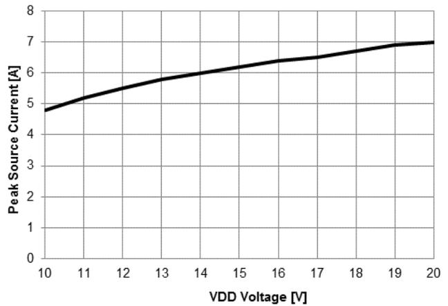
Figure 7. Sourcing Current vs. Operating Voltage ( $V_{DD}$ )
