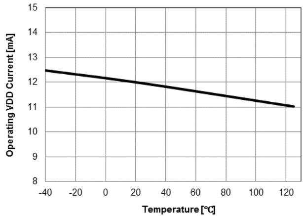
Figure 9. Operating Current ( $I_{DD}$ ) vs. Temperature
