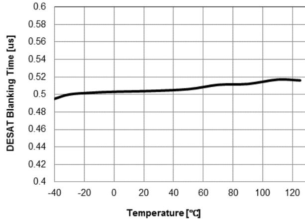
Figure 21. Desaturation Blanking Time ( $t_{DEL, DESAT}$ ) vs. Temperature
