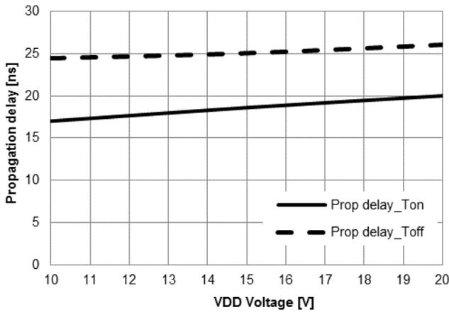
Figure 6. Propagation Delay Time vs. Operating Voltage ( $V_{DD}$ )
