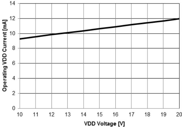
Figure 4. Operating Current ( $I_{DD}$ ) vs. Operating Voltage ( $V_{DD}$ )
