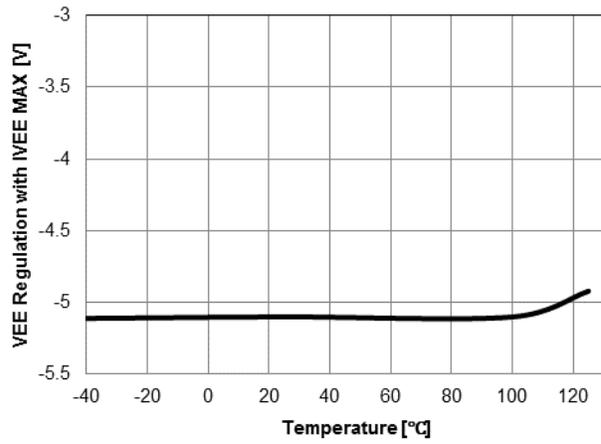
Figure 17. VEE5 Regulated Voltage with  $I_{VEE,MAX}$  vs. Temperature
