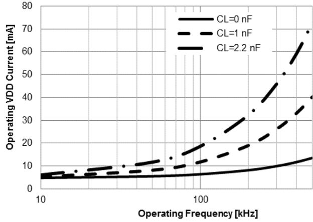
Figure 5. Operating Current ( $I_{DD}$ ) vs. Operating Frequency
