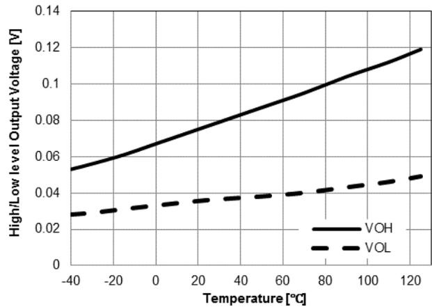
Figure 25. XEN Logic Output Voltage vs. Temperature
