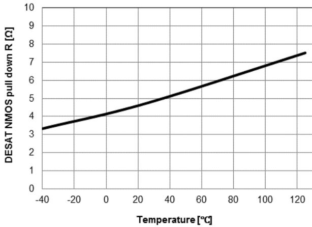
Figure 22. DESAT Pull Down Resistance ( $R_{DON,DESAT}$ ) vs. Temperature
