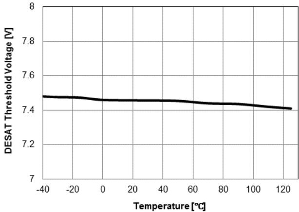
Figure 20. DESAT Threshold Voltage ( $V_{TH,DESAT}$ ) vs. Temperature
