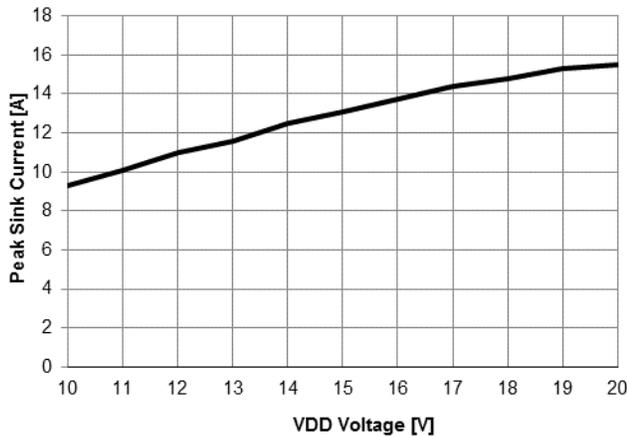
Figure 8. Sinking Current vs. Operating Voltage ( $V_{DD}$ )
