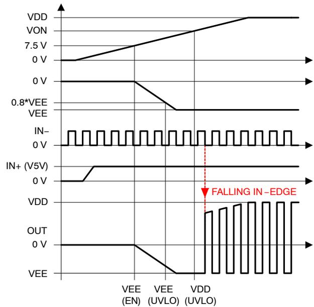
Figure 32. Inverting start-up logic
