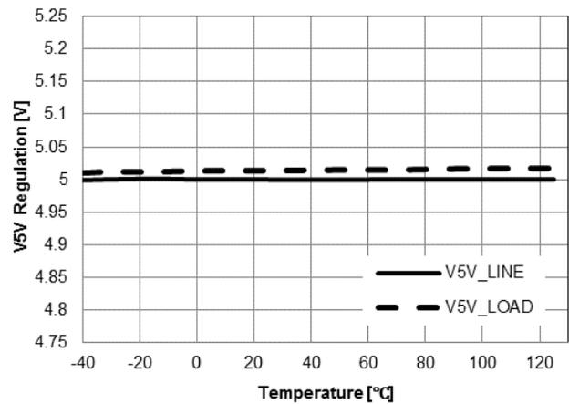
Figure 15. 5 V Regulated Output Voltage (V5V) vs. Temperature
