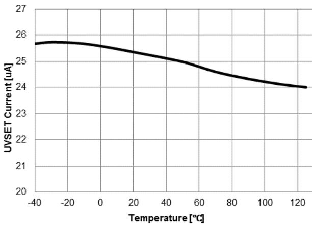
Figure 14. UVSET Current ( $I_{UVSET}$ ) vs. Temperature
