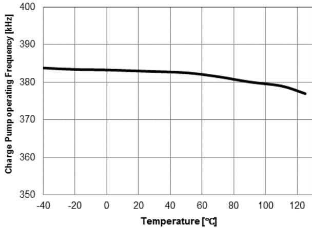
Figure 18. Charge Pump Operating Frequency ( $f_{osc}$ ) vs. Temperature
