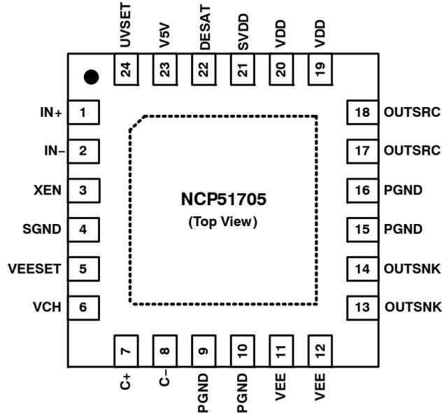
Figure 3. Pin Assignments – 24 Leads QFN (Top View)
