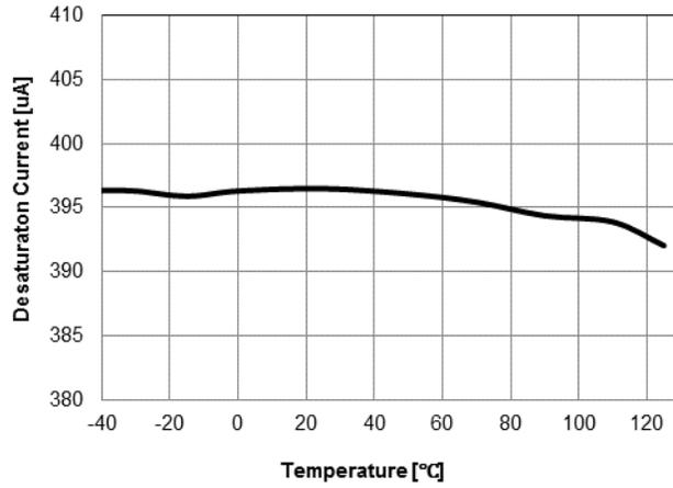
Figure 19. Desaturation Current ( $I_{DESAT}$ ) vs. Temperature
