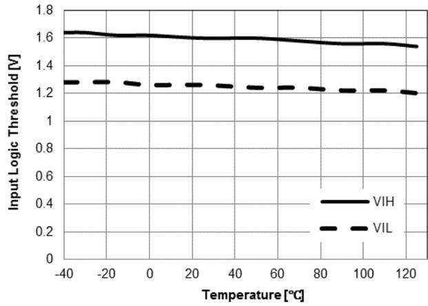
Figure 23. Input Logic Threshold Voltage vs. Temperature
