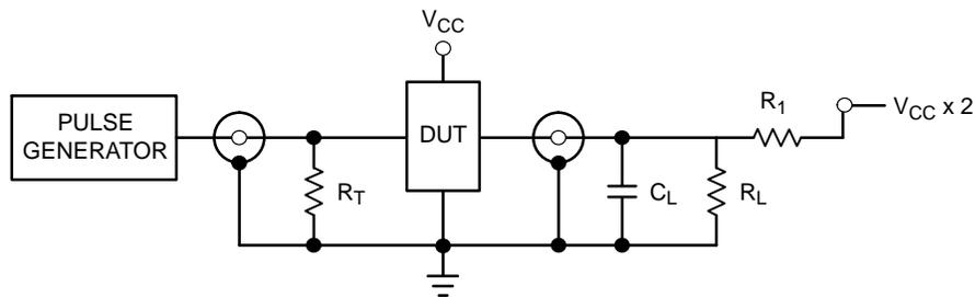
$R_T = Z_{OUT}$  of pulse generator (typically 50 Ω)
