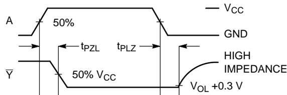
Figure 3. Switching Waveforms
