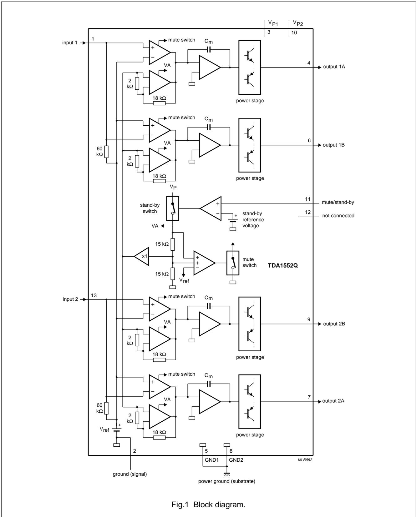
Fig.1 Block diagram.
