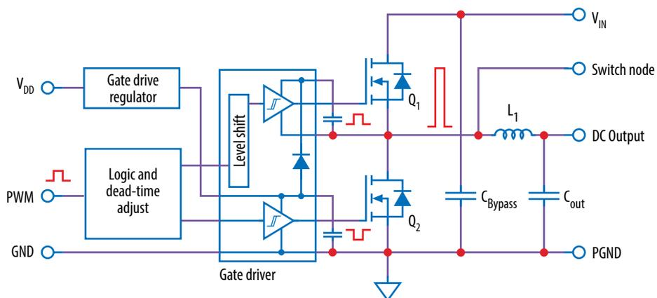
Figure 1: Block diagram of EPC9097 development board
