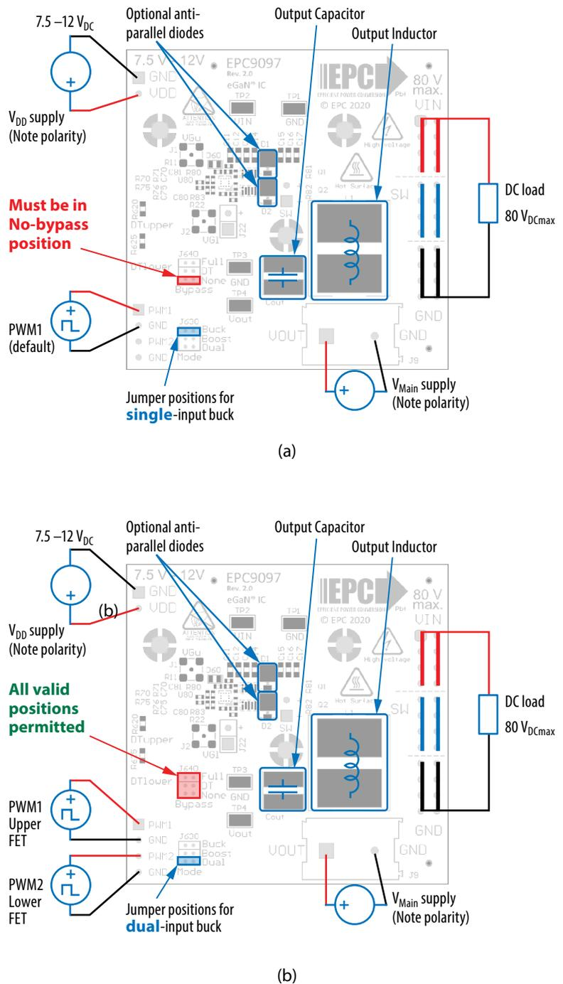
Figure 7: (a) Single-PWM input boost converter (b) Dual-PWM input boost converter configurations showing the supply, inductor, anti-parallel diodes, output capacitor, PWM, and load connections with corresponding jumper settings.
