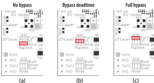
Figure 5: Bypass mode Jumper settings for J640
