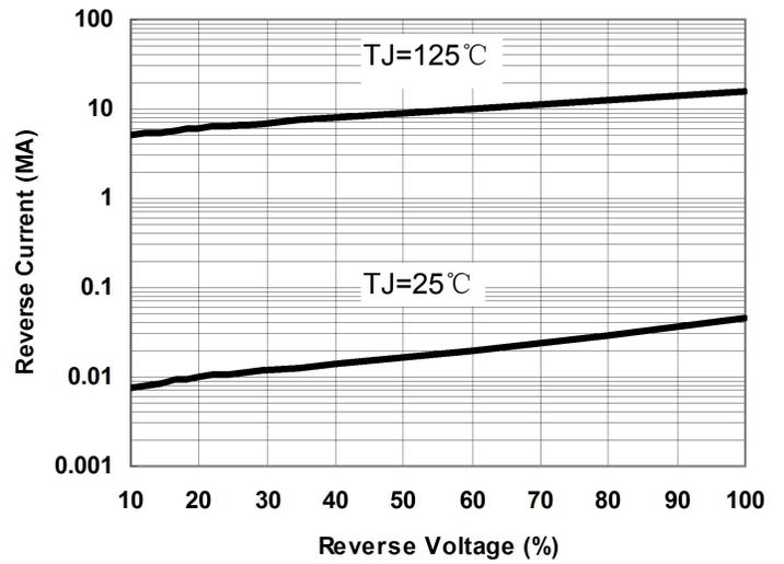
Fig.2-Typical Reverse Current
