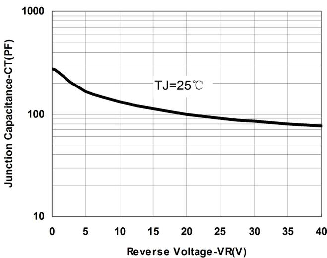
Fig.1-Typical Junction Capacitance
