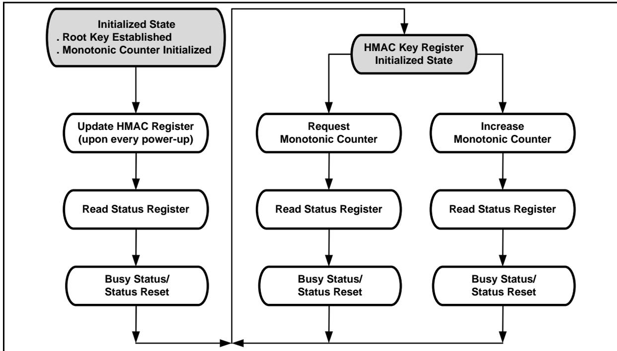
Figure 3b. W74M12FV Authentication Flash Operation Flow Diagram
