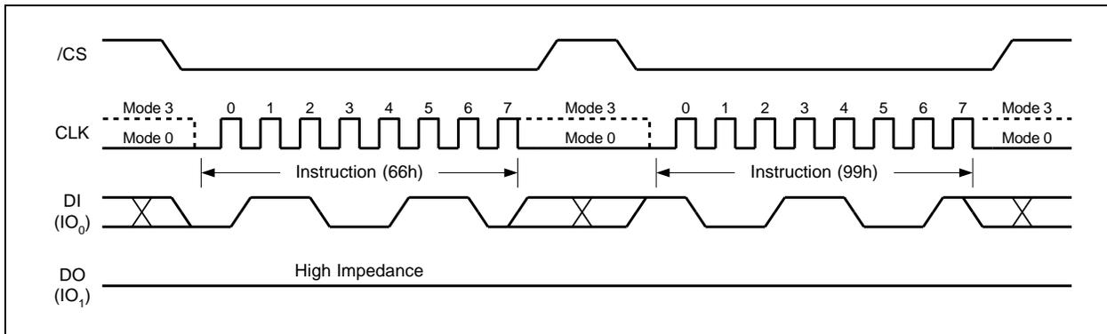
Figure 9. Enable Reset and Reset Instruction Sequence
