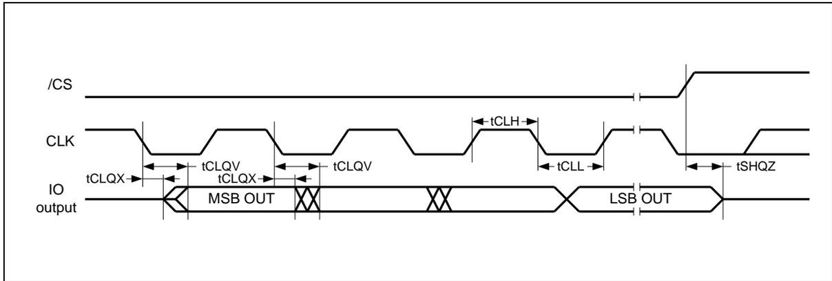
7.8 Serial Input Timing Diagram
