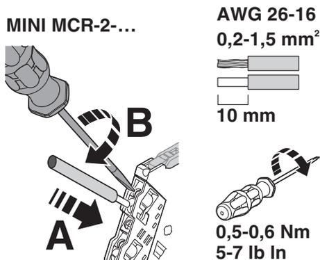
Figure 4 Screw connection
