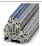
Feed-through terminal block, Cross section: 0.14 mm² - 6 mm², AWG: 26 - 10, Connection type: Screw connection, Width: 6.2 mm, Color: gray, Mounting type: NS 35/7,5, NS 35/15
