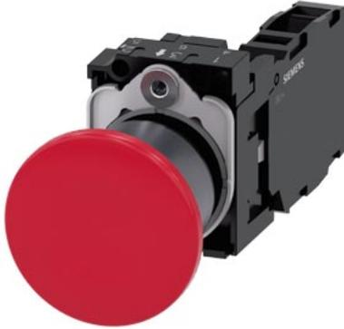
Mushroom pushbutton, 22 mm, round, plastic with metal front ring, red, 40mm, latching, pull-to-unlatch mechanism, with holder, 1 NO+1 NC, screw terminal, Z=20-unit packaging
